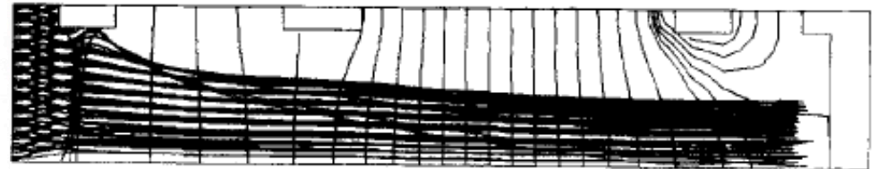
FIG. 4. Ion trajectories and potential distributions for a converged solution to Eqs. (9)–(12) showing the source-plasma sheath and nonlinear aberrations near the plasma electrode: S = 0.75 , \Gamma = 4 , and j = 0.45j_0 .
