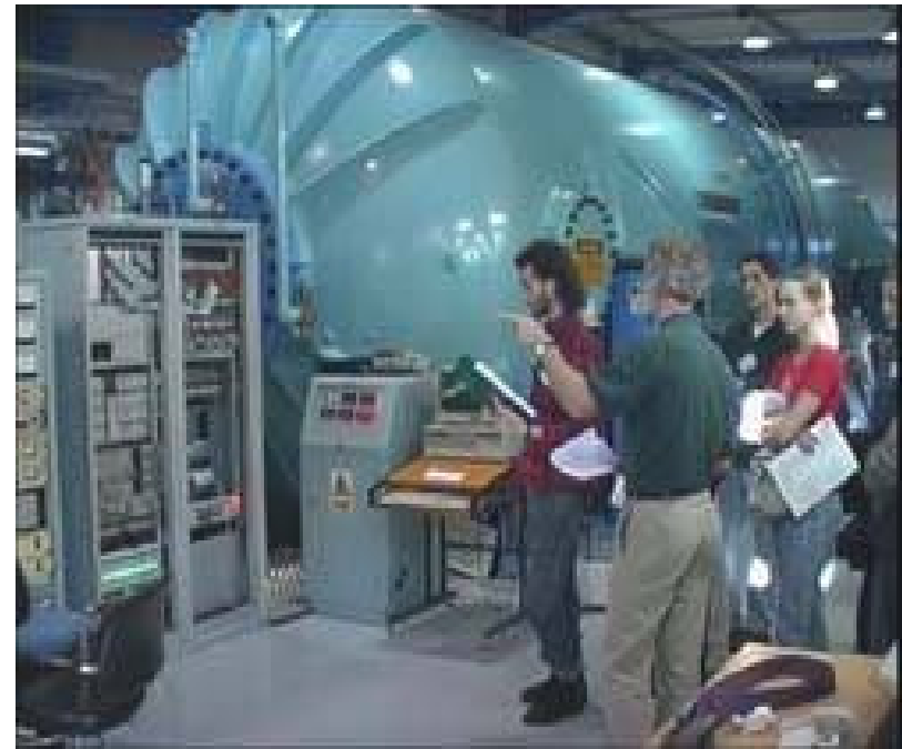
ANTARES Tandem Accelerator – 10MV
