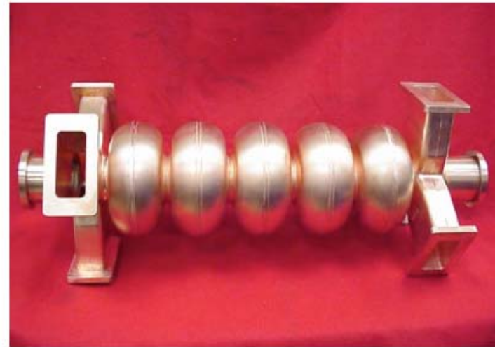
Figure 2: Copper five-cell model of the high-current cavity with waveguide end groups.
