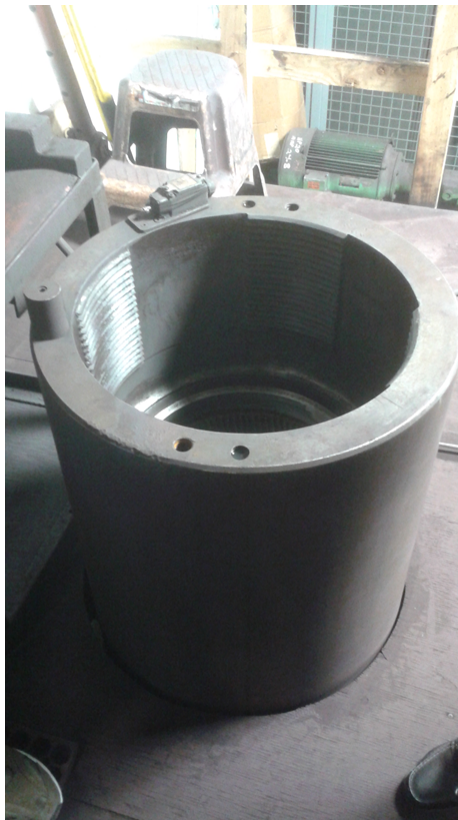
Figure 3.2: The canon at National Magnetics used to press the garnet powder into blocks.
