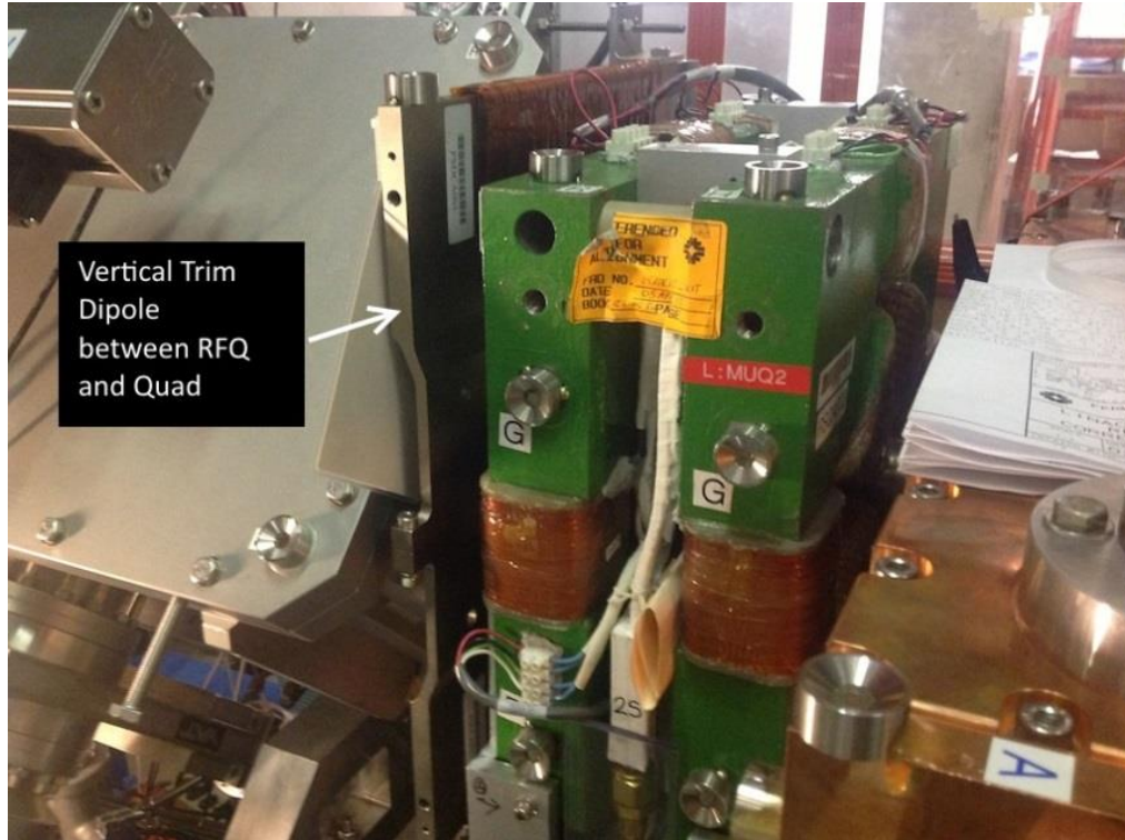
Figure 23: A dipole trim magnet was designed to fit in the small space between the RFQ and first MEBT quadrupole.
