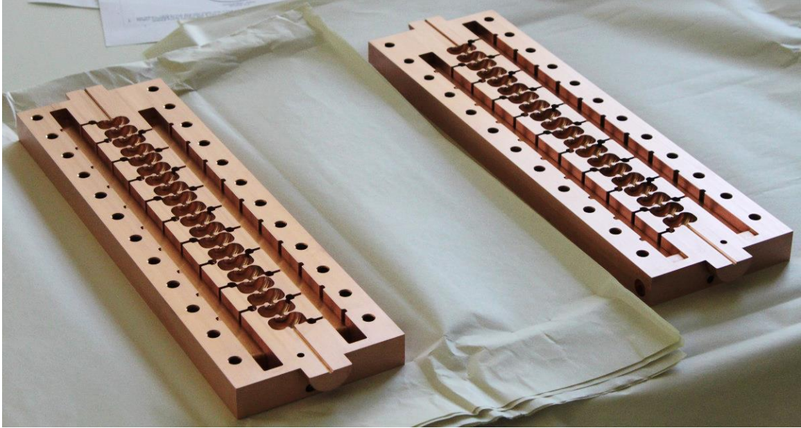
Figure 1-6: Distributed coupling accelerator from Dymenso. A single brazing plane runs the entire length of the accelerator, and two tuning pins per cell (not shown) allow for frequency tuning. Photo courtesy of Dymenso LLC and Phillip Borchard.
