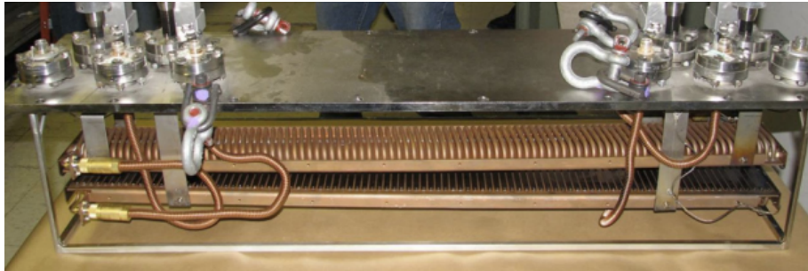
Figure 1.14: LANSCE slow-wave chopper [1].
