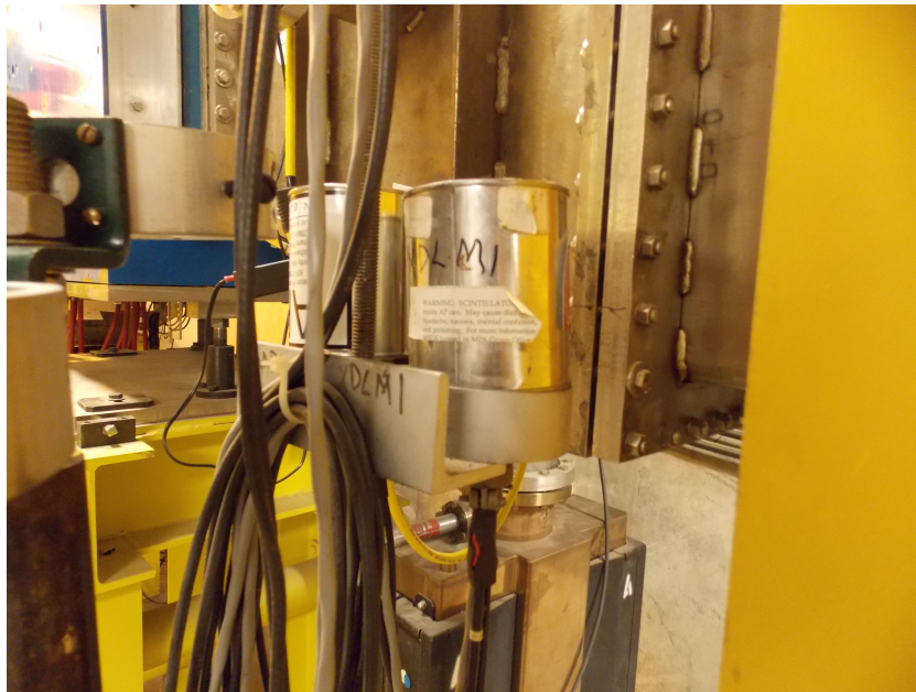
Figure 1.20: LANSCE activation protection (AP) and loss monitor (LM) scintillation detectors.
