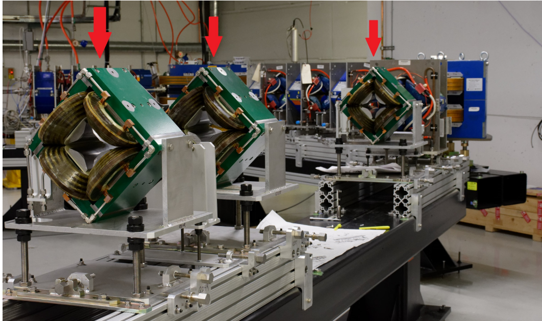
Figure 1.2: Picture of EMQD-280-709 quadrupole magnet for IOTA at Fermilab.
