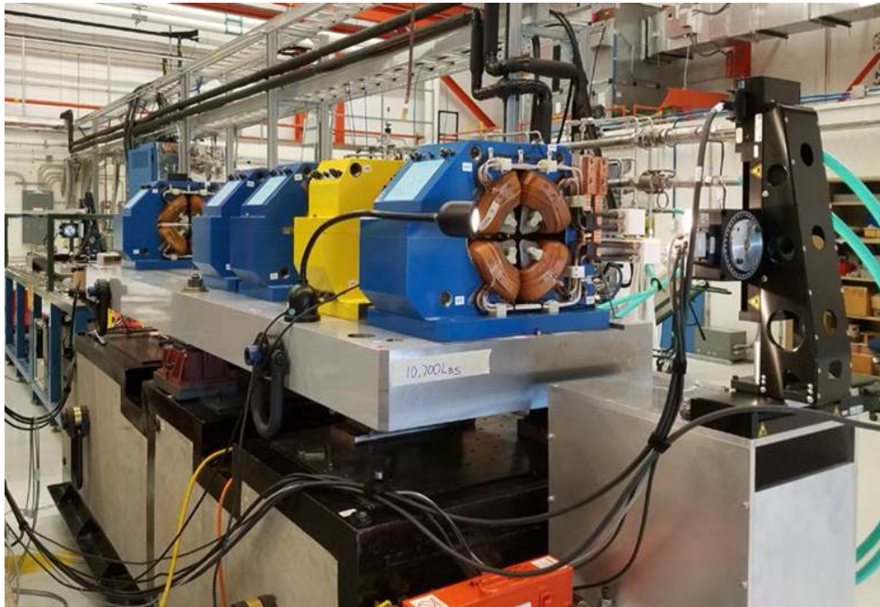
Figure 2.8: APS quadrupoles under alignment using ANL rotating wire [6].
