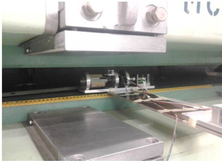
Figure 2.3: Rotating coil probe inside 1T reference dipole [4].
