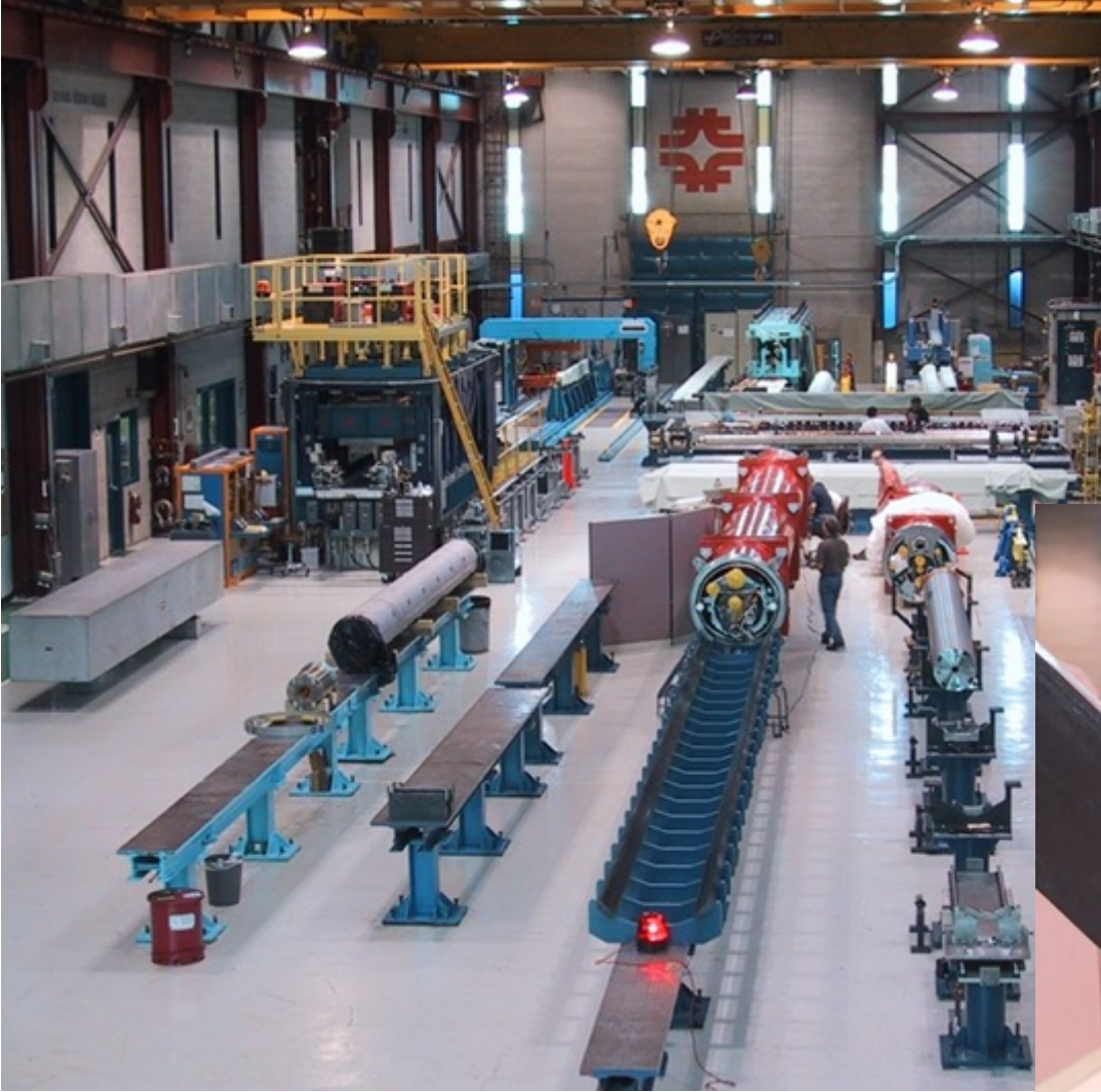
Assembly tooling for LHC IRQ magnets
