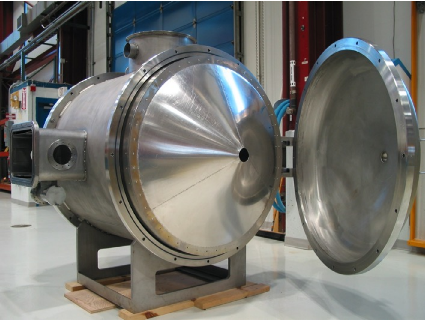
Spoke cavity test cryostat magnetic shield
