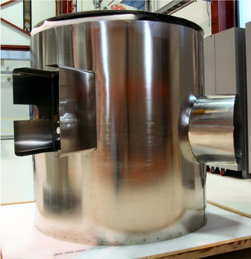
Spoke cavity test cryostat magnetic shield
