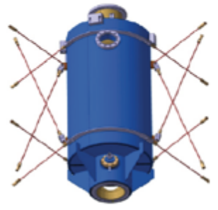
Figure 4.120: Helium vessel with hanging rod
