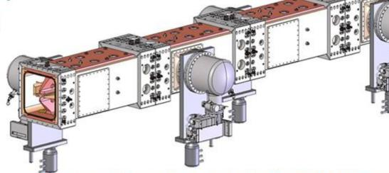
CAD model of assembled 4-module PXIE RFQ design concept
