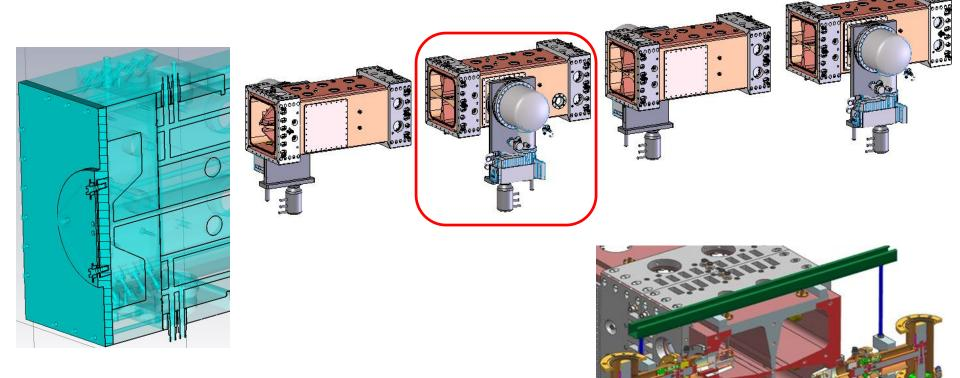
**Tuner at one end of the RFQ.** 50 mm protrusion, frequency shift is 45 kHz.
