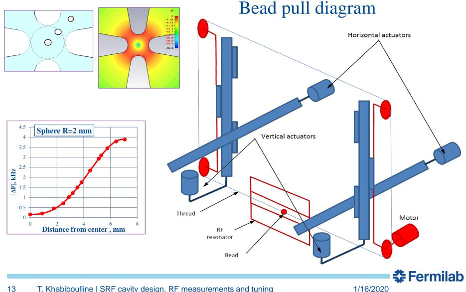
Positioning error can be compensated by averaging of measurements in all 4 quadrants  $df(x+dx, y+dy) \approx c \cdot f(x, y) + \alpha(x, y) \cdot dx + \beta(x, y) \cdot dy$ dB  $x = y \Longrightarrow \alpha(x, y) = \beta(x, y)$ dy  $\alpha(-x, y) = -\alpha(x, y); \alpha(x, -y) = -\alpha(x, y) \stackrel{dx}{=}$  $\beta(-x, y) = -\beta(x, y); \beta(x, -y) = -\beta(x, y)$ df(x+dx, y+dy)+df(-x+dx, y+dy)+ $df(x+dx,-y+dy) + df(-x+dx,-y+dy) \approx 4c \cdot f(x,y)$
