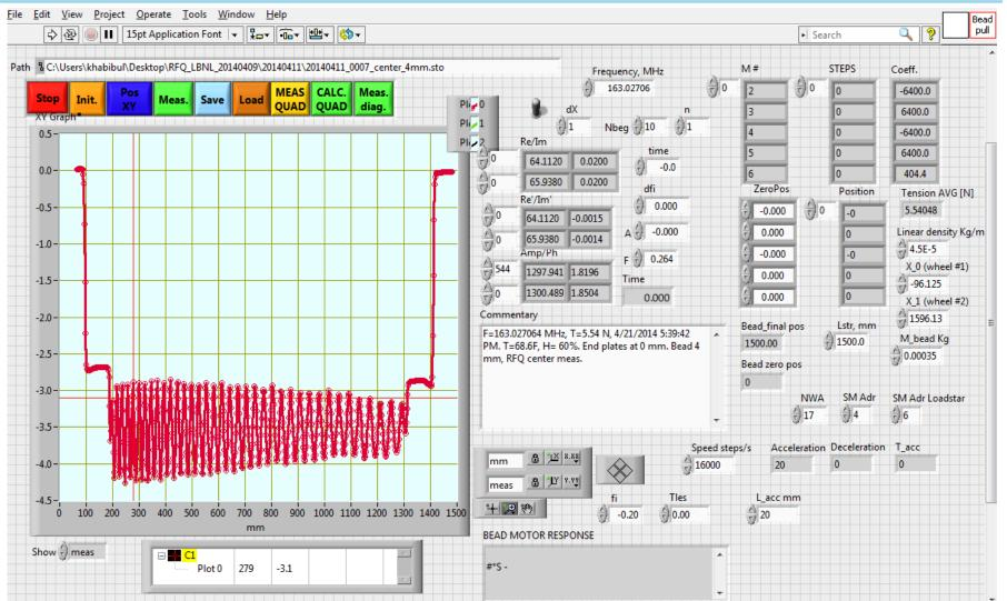
Program allow to position bead in any location near cavity center and measure field flatness. Multiple passes and post processing is included.
