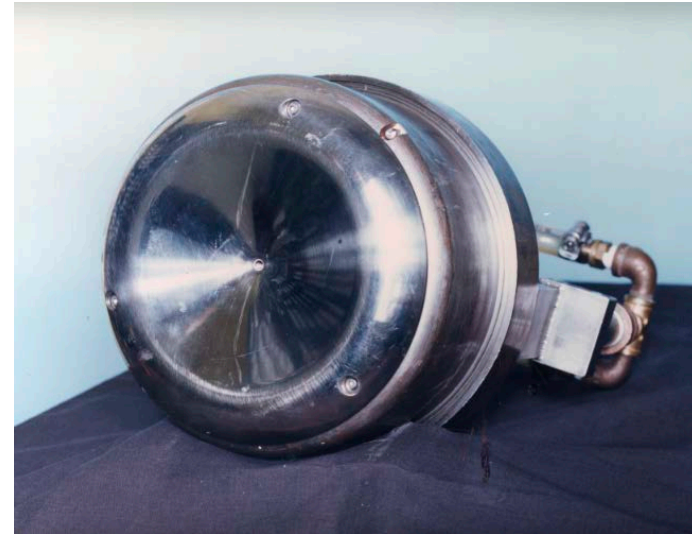
Side view of assembled LANSCE duoplasmatron ion source with Pierce electrode.
