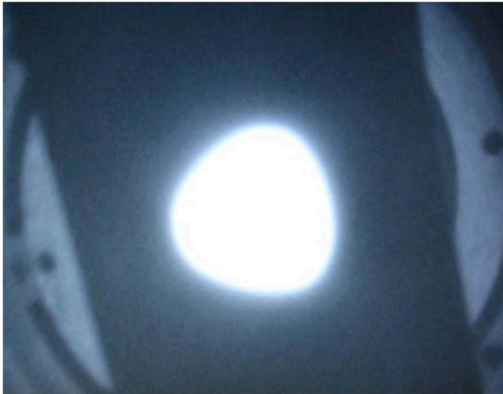
Image of a triangular He + beam 80 cm after extraction. (D.Winklehner et al, 2010 JINST 5, P1 2001)
