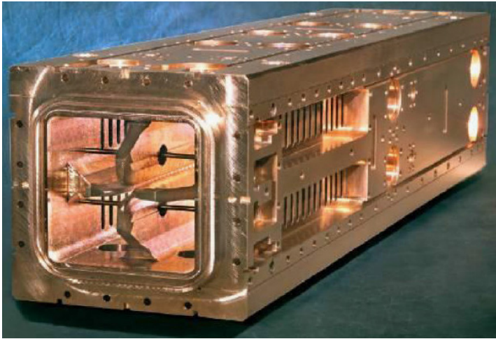
SNS 4-vane RFQ with \pi -mode stabilizers. Total length is 3.72 m, 4 modules. 402.5 MHz, 40 mA H^- , 65 keV to 2.5 MeV
