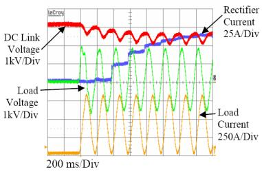
Figure 4: First few cycles after turn on.
