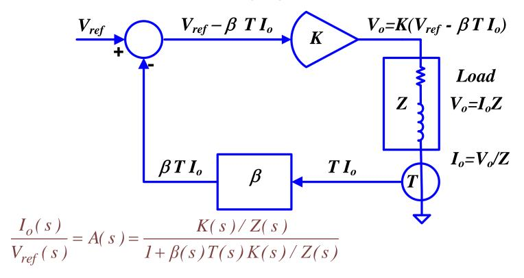
Very simply:  $1+\beta(s)$  T(s)K(s)/Z(s) must not =0 or approach 0 (avoid singularity)  $\beta(s)$  T(s) K(s)/Z(s) must not =-1 in order to avoid oscillations  $|\beta|e^{j\alpha}|T|e^{j\beta}/K|e^{j\chi}/|Z|e^{j\phi}=|\beta||T||K||1/Z|e^{j(\alpha+\beta+\chi-\phi)}$   $|\beta||T||Z||1/K|\neq 1$  when  $\alpha+\beta+\chi-\phi=\pm 180^{\circ}$
