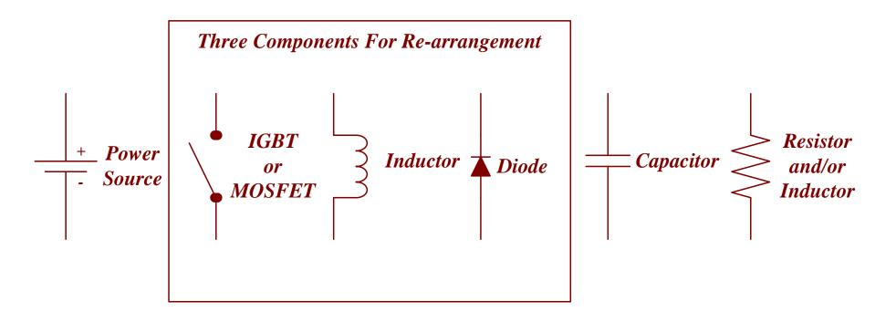
Most fundamental switchmode converter topologies are constructed by rearranging the three components
