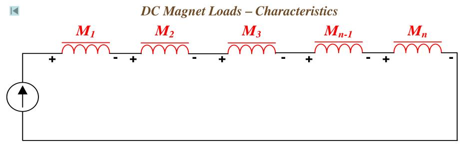
String (series-connect) magnets for economy when there are no special optics requirements. The current in each series-connected magnet is the same.
