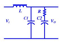
$$T = \frac{s R C_2 + 1}{s^3 R L C_1 C_2 + s^2 L(C_1 + C_2) + s R C_2 + 1}$$
