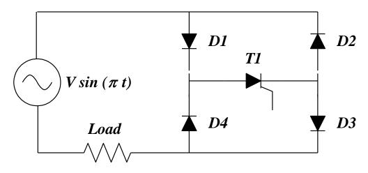
Assume ideal components in the phase-controlled circuit above. For a purely resistive load:
