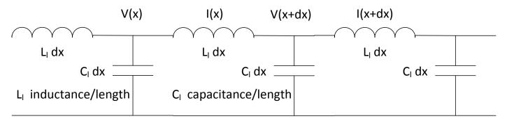
$$V(x + dx, t) - V(x, t) = -L_l dx \frac{\partial I(x, t)}{\partial t}$$
