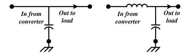
• L filters consist of one inductive element and one capacitor. One disadvantage is that the inductor element in smaller filters consists of a ferrite bead that will saturate and lose effectiveness at larger load currents
