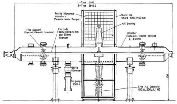
Fig.2 Separator chamber.
