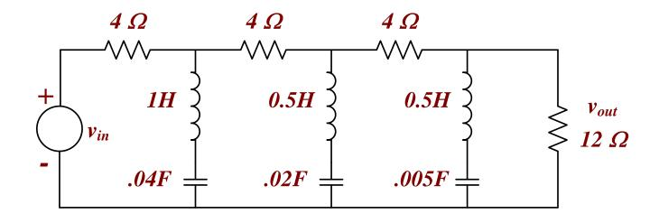
$$h(t) = \frac{v_{out}(t)}{v_{in}(t)} \qquad H(j\omega) = \frac{V_{out}(j\omega)}{V_{in}(j\omega)}$$
