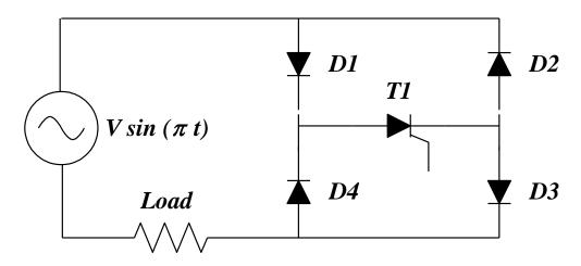
Assume ideal components in the phase-controlled circuit above. For a purely resistive load:
