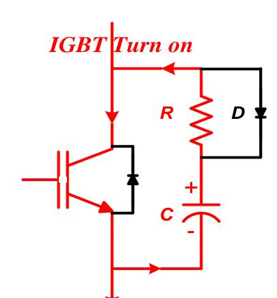
• When the IGBT turns on, the capacitor C, discharges through R and the IGBT
