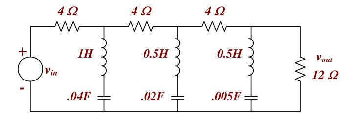
$$H(j\omega) = \frac{V_{out}(j\omega)}{V_{in}(j\omega)}$$
