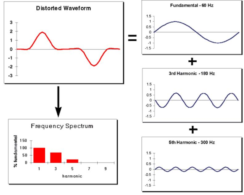
A waveform v(t) was analyzed and found to consist of 6 components as shown here.
