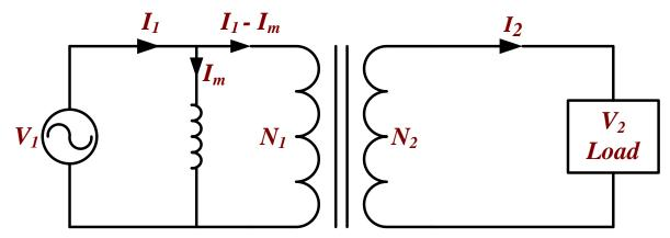
Secondary winding turns cut by the common flux produce a voltage with the same volts per turn as the driving primary turns
