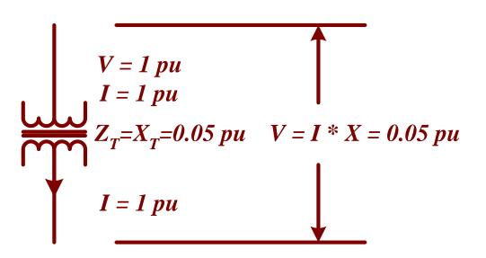
Referring to the one-line diagram below, determine the line currents in the:
