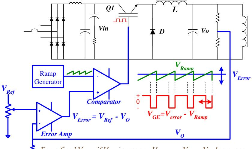
For a fixed  $V_{Ref}$  if  $V_O$  increases,  $V_{Error} = V_{Ref} - V_O$  decreases accordingly. The pulse width will decrease to make  $V_O = V_{Ref}$
