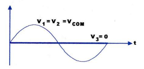
• Produced as a result of circuit imbalances, currents produced by simultaneous high frequency voltages on (+) and (-) lines capacitively coupled to ground
