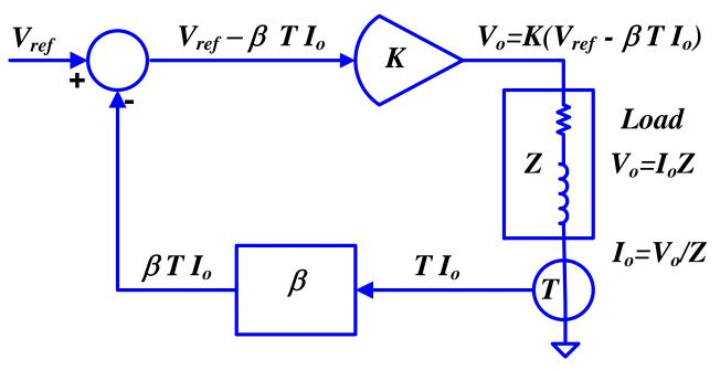
The feedback loop ensures the output always follows the input
