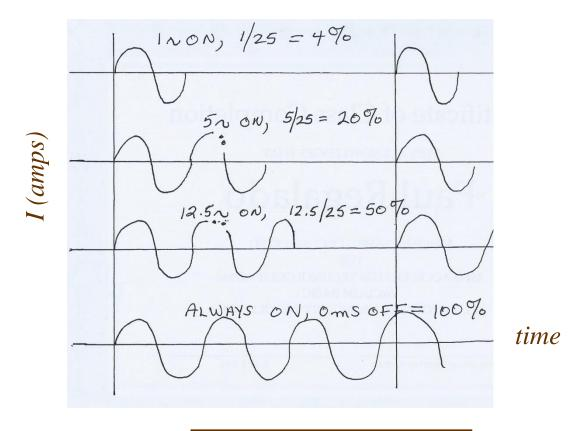
$$I_{RMS} = \frac{\sqrt{\frac{1}{\omega T} \int_{0}^{\omega T} (I_{pk} \sin \omega t)^{2} d\omega t}}{\frac{T_{on}}{T_{cycle}}}$$
