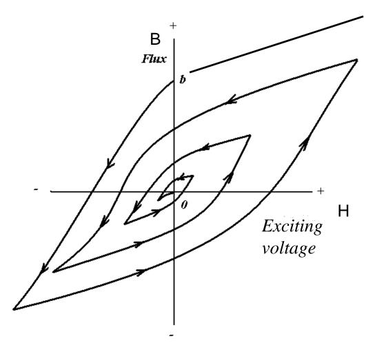
Removing residual magnetism from a ferromagnetic circuit by using decreasing excitation
