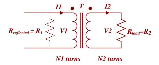
$$R_{1} = \frac{V_{1}}{I_{1}} = \frac{\frac{N_{1}}{N_{2}}V_{2}}{\frac{N_{2}}{N_{1}}I_{2}} = \frac{N_{1}V_{2}}{N_{2}} * \frac{N_{1}}{N_{2}I_{2}}$$
