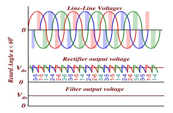
For  $0 \le \alpha \le \frac{\pi}{3}$  where  $\alpha$  is the gate trigger retard angle and conduction is continuous
