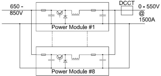
Figure 1: Dipole Converter Topology.
