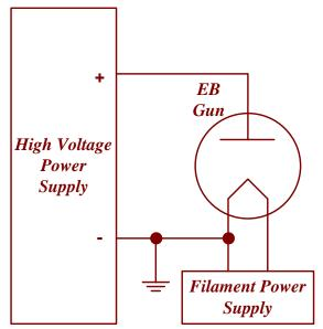
If work surface (anode) is easy to insulate - float at HV. Put filament at ground potential.
