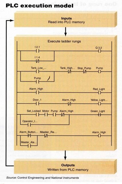
Ladder diagrams evolved in the 1960s when the automobile industry needed a more flexible and self-documenting alternative to relay and timing cabinets. A microprocessor was added and software designed to mimic the relay panels.
