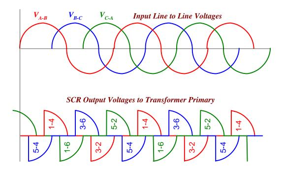
$$V_{RMS} = \sqrt{\frac{1}{\omega T} \int_{\alpha}^{\omega T} \sqrt{2} V_{LL} \sin^2 \omega t \ d\omega t}$$
