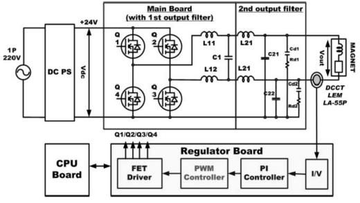
Figure 4: Circuit diagram of bipolar MPS.
