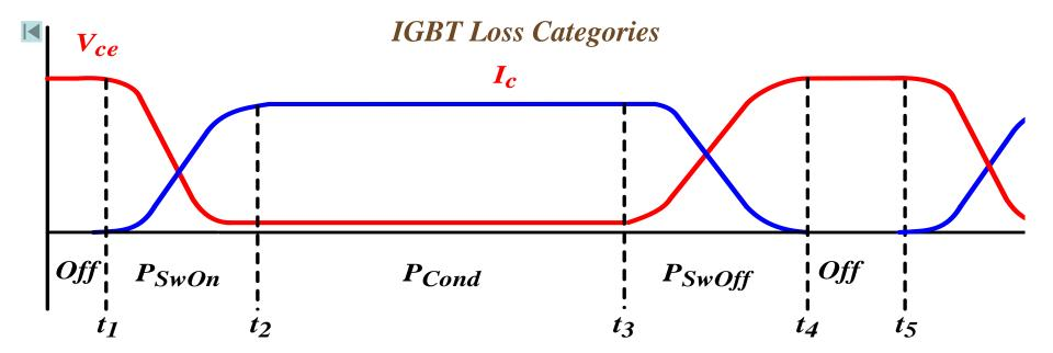
$$P_{SwOn} = \frac{1}{t_5 - t_1} * \int_{t_1}^{t_2} v_{CE}(t) * i_C(t) * dt$$
