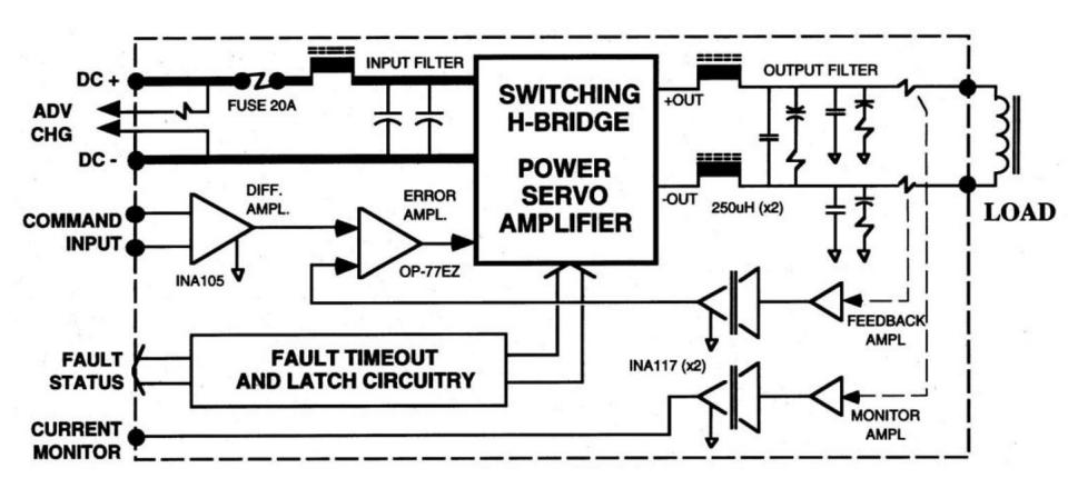
Figure 1.3. MCOR12 Block Diagram.
