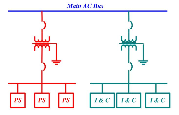
• Separate noisy power supplies from sensitive I & C loads by Faradayshielded transformers to attenuate common mode noise
