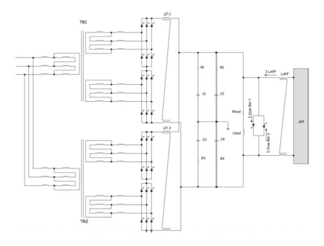
Figure 2: Topology of CNAO synchrotron power supply.
