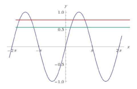
$$I_{AVG}(DC) = \frac{1}{\omega T} \int_0^{\omega T} I_{pk} \sin \omega t \, d\omega t$$
