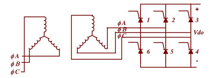
The current on the primary leg of the transformer, due to the YY winding is
