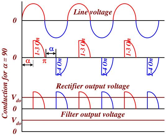
$$V_{do} = \frac{1}{T} \int_{t}^{T} v_{LL}(t) dt = \frac{1}{T} \int_{t}^{T} \sqrt{2} V_{LL} \sin \omega t \ dt = \frac{1}{\omega T} \int_{\alpha}^{\omega T} \sqrt{2} V_{LL} \sin \omega t \ d\omega t$$
