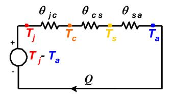
$T_a = Ambient \ air \ or \ cooling \ water \ inlet \ temperature \ (^{O}C)$
