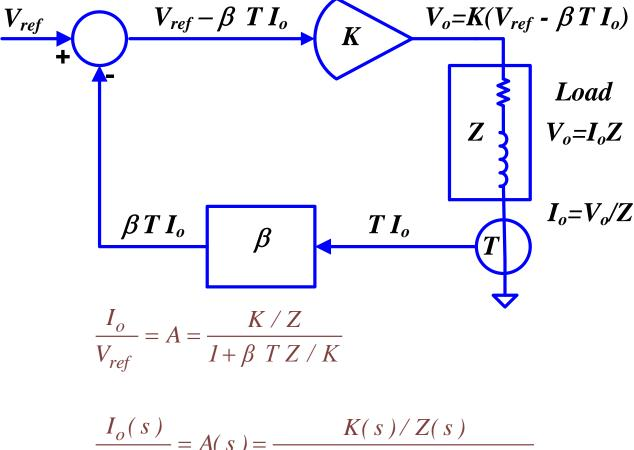
$$\frac{I_o(s)}{V_{ref}(s)} = A(s) = \frac{K(s)/Z(s)}{1+\beta(s)T(s)Z(s)/K(s)}$$
