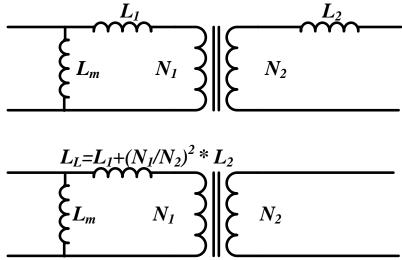
• If the secondary is shorted the "percent impedance" is the drive voltage divided by the rated input voltage with rated load current flowing
