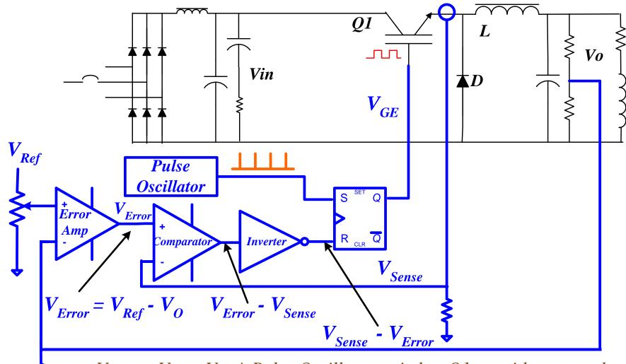
$oldsymbol{V_{Error}} = V_{Ref} - V_O$ . A Pulse Oscillator switches Q1 on with every pulse. L current is converted to a voltage by a sense resistor. The L current builds up to the threshold set by the error voltage which then turns off Q1 in order to keep the output voltage or current constant.
