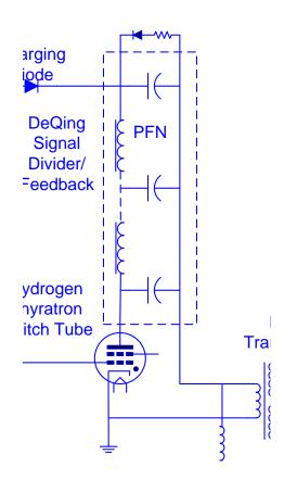
The PFN is typically tuned to the impedance of the load in order to reduce voltage and current reflections. The effective output voltage at the load obeys the voltage divider law and is effectively
