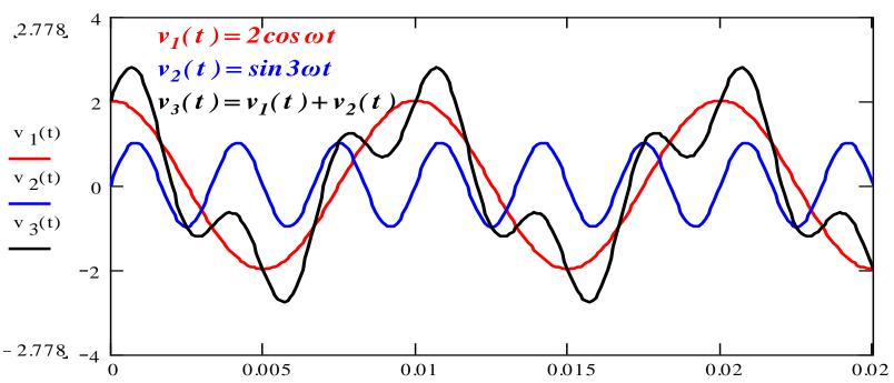
Trigonometric forms of the Fourier Series
