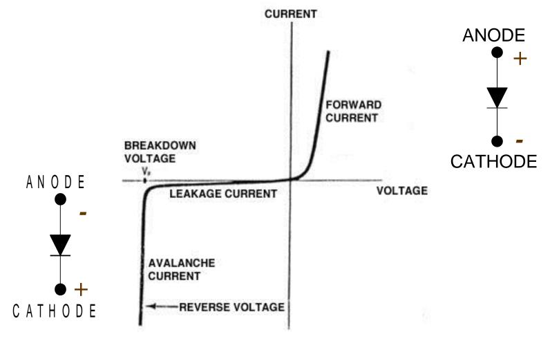
In the reverse direction, there is a small leakage current up until the reverse breakdown voltage is reached
