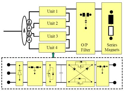
Figure 1: Booster dipole power circuit.
