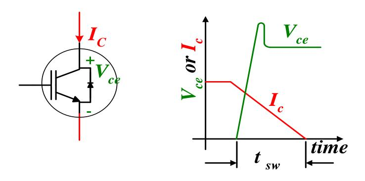
$$P_{SwOff} = \frac{1}{T} \int_{0}^{t_{Sw}} v_{CE}(t) i_{C}(t) dt$$
