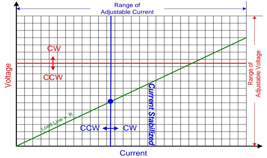
Constant Current Mode. The power supply will operate in this mode whenever the voltage demanded by the load is less than that defined by the front panel voltage control. The output current is set by the front panel current control. The output voltage is set by the load resistance and the I set.
