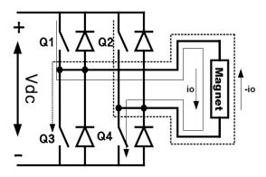
Figure 1: Bipolar MPS operation of full-bridge four-quadrant DC/DC converter.
