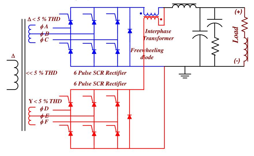
Transformer phases and SCR firing sequence are the same as shown for the series-connected bridges
