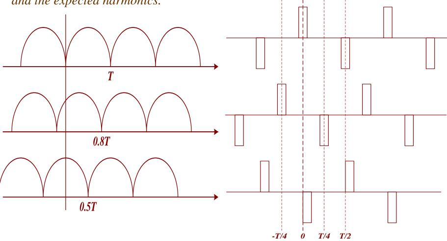
Signal Total Harmonic Distortion (THD): The ratio of the square root of the summed squares of the amplitudes of all harmonic frequencies above the fundamental frequency to the fundamental frequency
