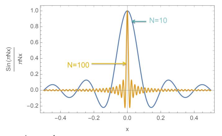
$\frac{\Delta \omega_k}{\omega_k} = \pm \frac{1}{kN_p}$  first zeros near the origin define the width of the peak.
