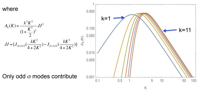
Undulator parameter K should be between 1 to 4
