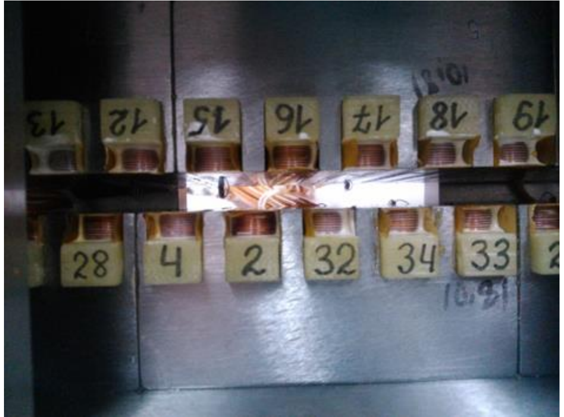
Position of the frames. Upper and bottom frames are shifted of \frac{1}{2} period
