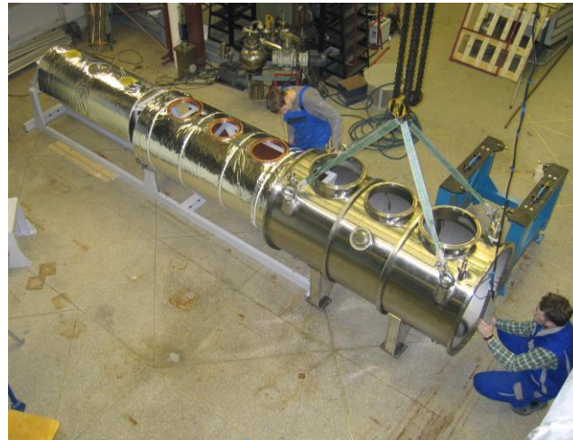
Wiggler assembling on site
