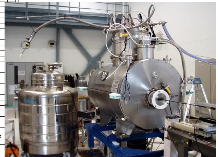
Magnetic field measurements of 10 T WLS
