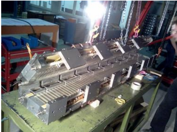
Open magnet for vacuum chamber installing
