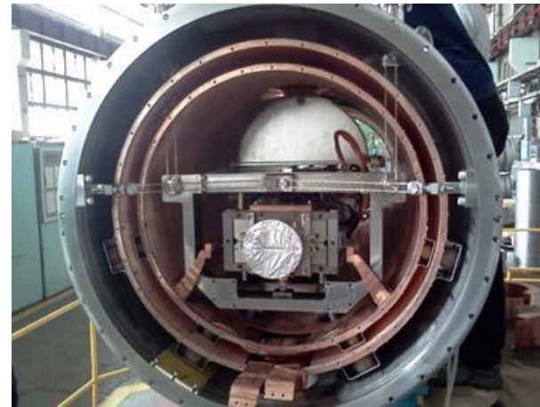
The magnet inside the cryostat
