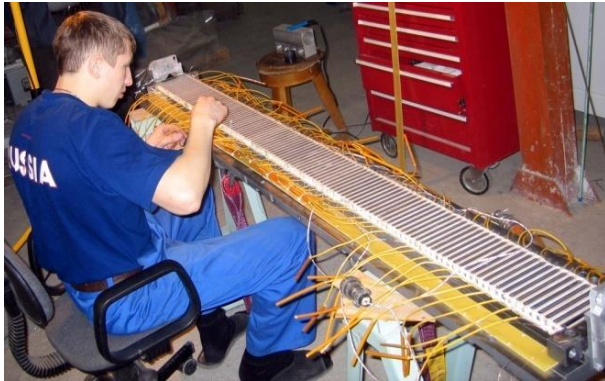
Magnet array of horizontal racetrack type poles (example of 30 mm period SC 2.1T wiggler)
