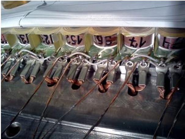
Heat sinks of the magnet poles
