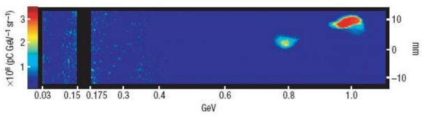
Density 4.3 10<sup>18</sup> cm<sup>-3</sup> Laser Power > 38 TW (73 fs) to 18 TW (40 fs)  $E = 1.0 \pm -0.06 \text{ GeV}$   $\Delta E = 2.5\% \text{ r.m.s}$   $\Delta \theta = 1.6 \text{ mrad r.m.s.}$ Q = 30 pC charge
