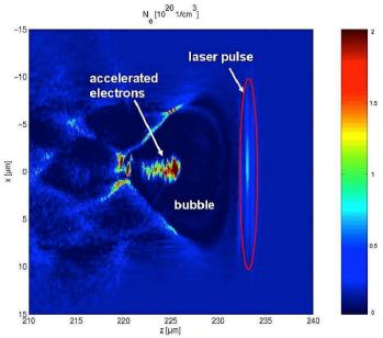
Laser plasma wakefield accelerators demonstrated the possibility of generating GeV beam with promising electron beam qualities
