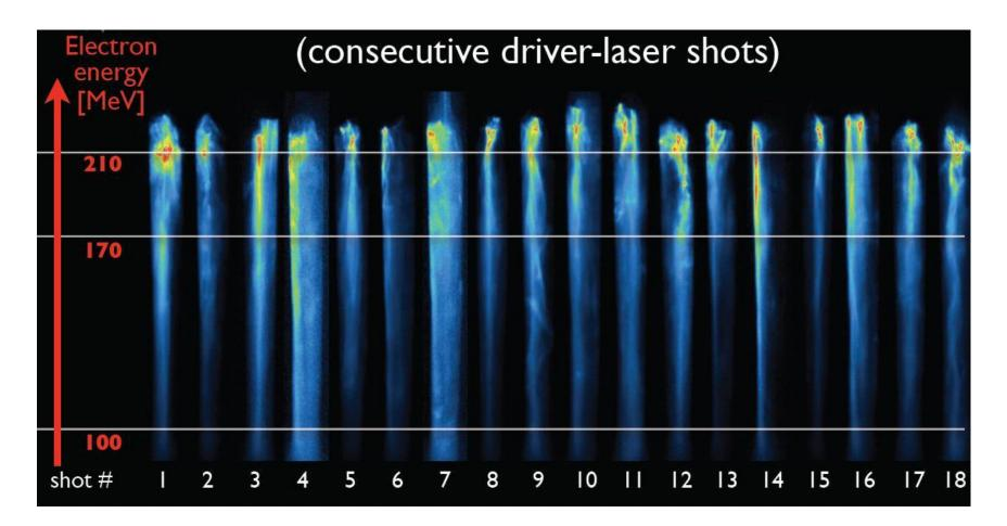
Stability of the electron beam quality is crucial for a successful FEL operation
