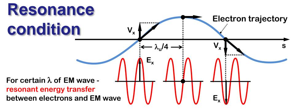
Condition for resonant energy transfer is that EM wave slips forward with respect to electron by  $\lambda$  /2 per half period of electron trajectory, i.e.
