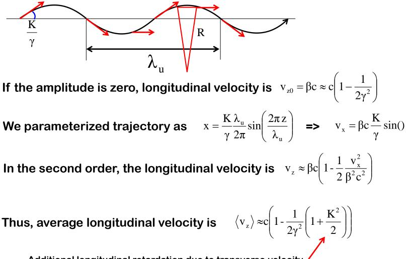
Additional longitudinal retardation due to transverse velocity
