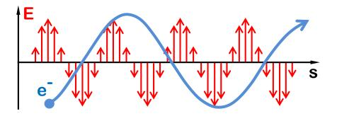
Energy exchange EM wave - electrons  $\frac{dW}{dt} = e \vec{E} \cdot \vec{v} \neq 0$  because  $\vec{v}_{\perp} \neq 0$
