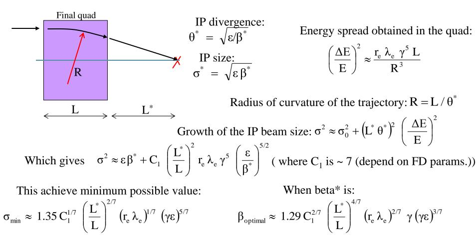
Note that beam distribution at IP will be non-Gaussian. Usually need to use tracking to estimate impact on luminosity. Note also that optimal  $\beta$  may be smaller than the  $\sigma_z$  (i.e cannot be used).
