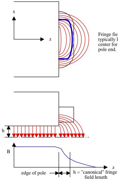
Fringe field length is typically longer in the center for an "unchamfered" pole end.
