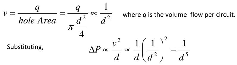
If the design hole diameter is increased, the required pressure drop is decreased dramatically.
