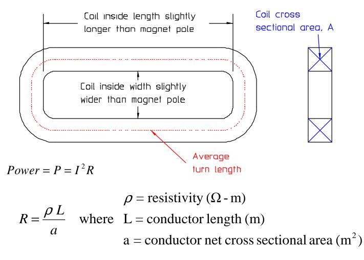
$L = N\ell_{ave}$  where N = number of turns in the coil. Na=fA where f = coil packing fraction.
