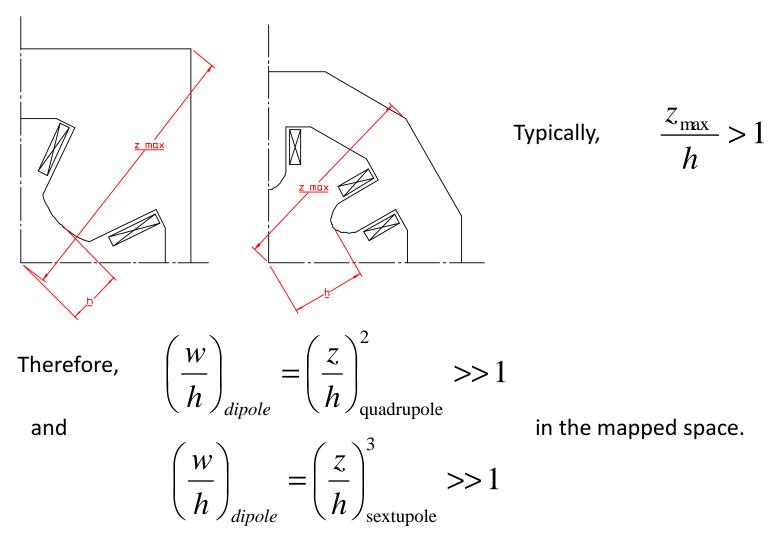
• When mapping from the quadrupole or sextupole geometries to the dipole space, the FEM computation is initially made in the original geometry and a vector potential map is obtained at some reference radius which includes the pole contour.
