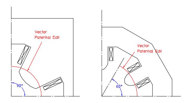
The vector potential values are then mapped into the dipole (w) space and used as boundary values for the problem.
