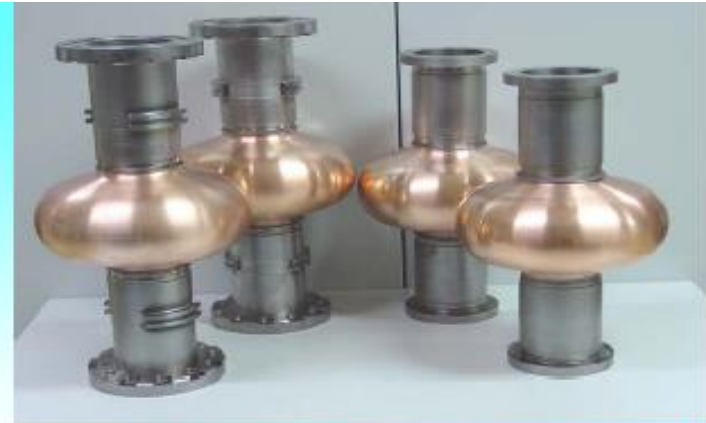
NbCu cavities hydroformed from explosively bonded tubes at DESY.
