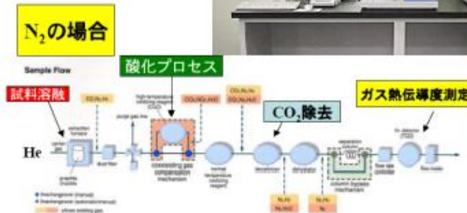
Gas analysis (Hydrogen, Oxygen, Nitrogen) : HORIBA
