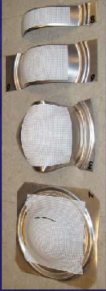
Aluminum alloy samples used in limit dome tests.
