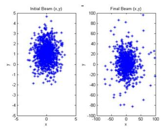
Figure 1.15: Distributions of muon positions in the beam at the start of the traversal of the iron, (left), and after complete traversal of the iron block (right). The scales are a factor of 20 different.
