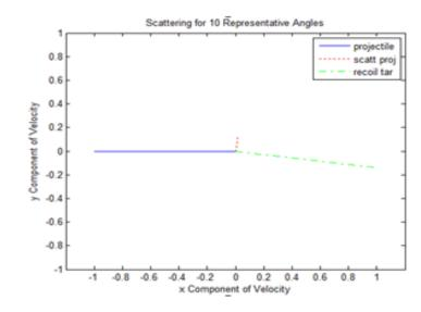
Figure 2.14: Scattering of a projectile and the recoil momentum and angle for the case of equal target and projectile mass. This is a snapshot of a movie covering several scattering angles.
