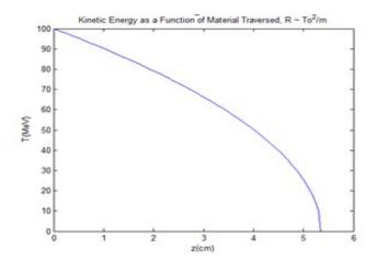
igure 7.16: Kinetic energy of a 100 MeV proton in water as a function of the distance avelled.
