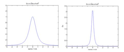
Figure 7.14 Transverse fields of a moving charge observed at the point x = d, y = 0 =z. At left the charge moves with  $\beta = 0.1$ , while at right it has velocity  $\beta = 0.95$ .
