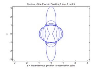
Figure 7.13: Contours of the electric field of a uniformly moving charge.
