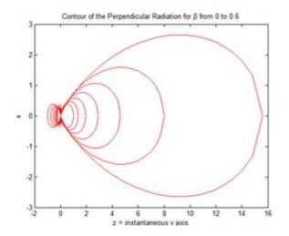
Figure 7.19: Perpendicular acceleration angular pattern as a function of the source velocity.
