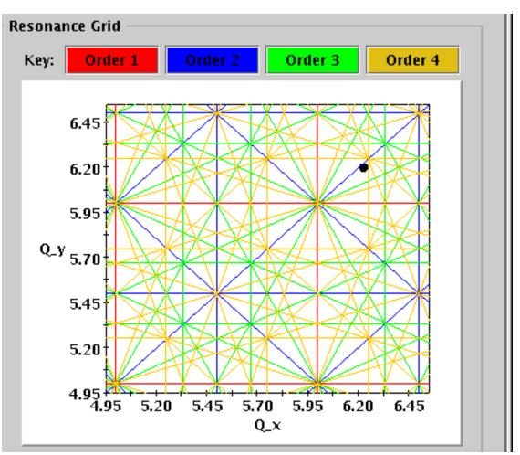
We could populate the diagram endlessly, but since resonances become weaker with increasing order gets, it's not necessary.
