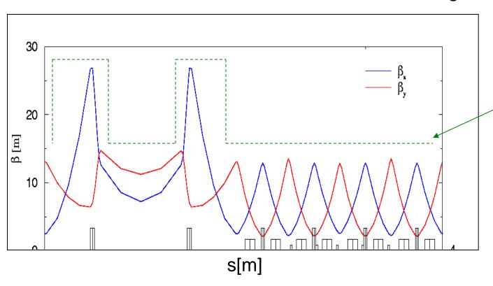
Beam pipe aperture scales with beta function.
