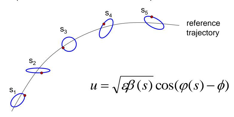
The motion of the particle in real space, u, is "quasi-harmonic".
