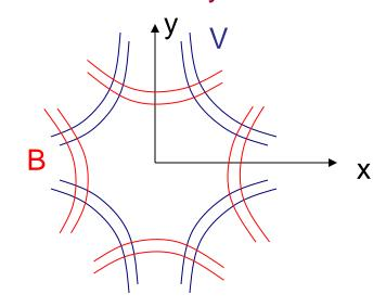
These are the equations for a normal quadrupole, which we derived earlier. We can associate the coefficient  $A_2$ - $B_2$  with the quadrupole strength, k.
