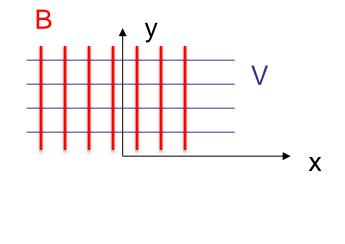
We find that n=1 gives a dipole field. The coefficient  $A_1$ - $B_1$  is the dipole strength found earlier ( $\kappa$ =1/ $\rho$ ). Note that for the normal case, only the vertical field (horizontal bending) is present.
