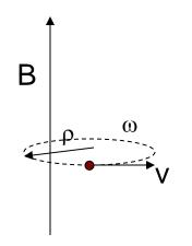
To find the direction of the force on the particle, use the right-hand-rule.
