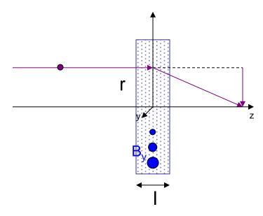
For a field which increases linearly with r, the resulting kick will also increase linearly with r.
