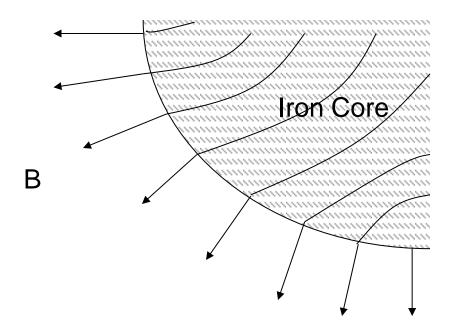
Magnetic lines may have both || and  $\perp$  path inside the material, but outside, only the field  $\perp$  to the surface survives. To get as strong of a field in the gap as possible, we should try to make the  $\perp$  piece inside as large as possible.
