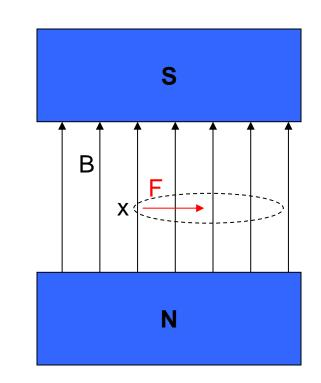
In an accelerator lattice, dipoles are used to *bend* the beam trajectory. The set of dipoles in a lattice defines the *reference trajectory*:
