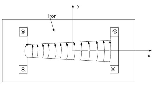
The B field in this magnet has both quadrupole and dipole components.
