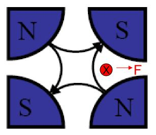
This magnet is horizontally defocusing. A distribution of particles in x would be defocused!
