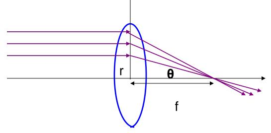
The farther off axis, the stronger the focusing effect! The dependence is **linear** for small x.
