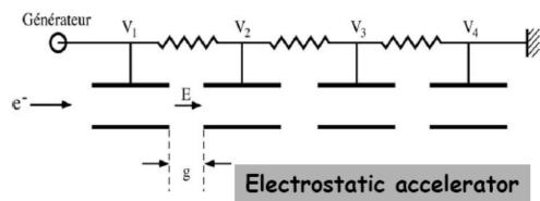
Accelerating column in electrostatic accelerator
