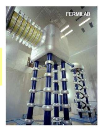
Modern Cockroft-Waltons are still used as proton injectors for linear accelerators
