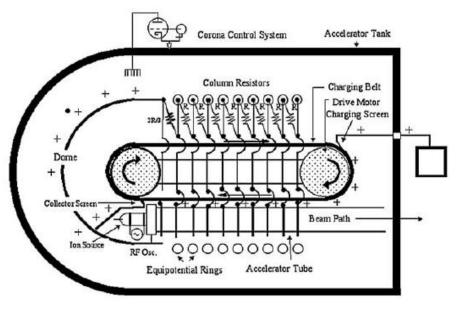
Fig. 6.2. A simple belt-charged accelerator
