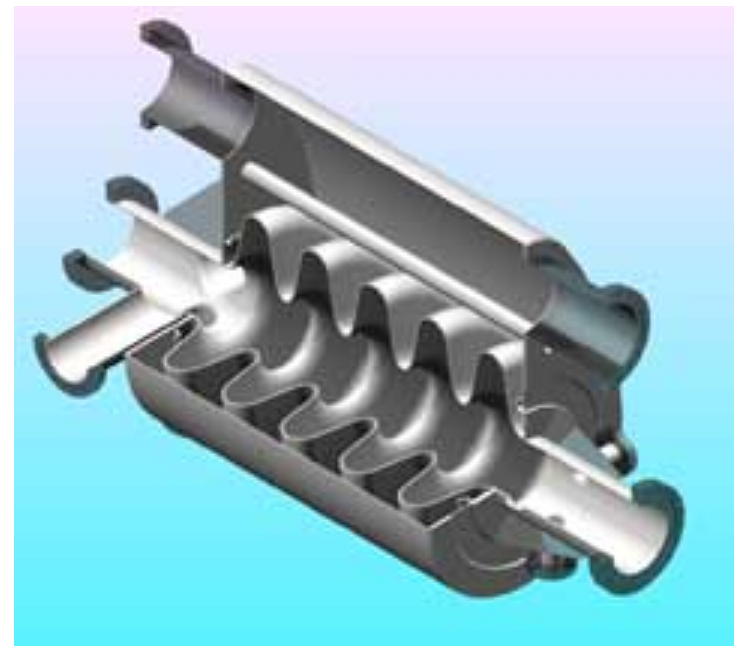
CAD drawing of a superconducting cavity elliptic cavity with 5 “gaps”
