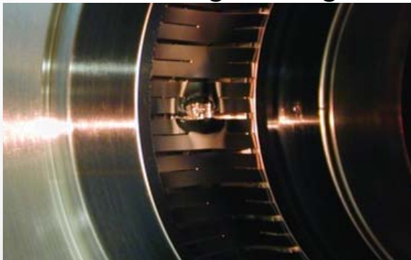
RF-shield fingers of gate valve
