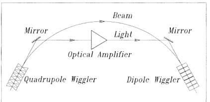
Cooling time  $\tau$  estimate  $\frac{\tau}{T} \approx \frac{N}{\Delta f} (c/l_b) \approx 2N_u$   $\tau$ : cooling time, c: spd of light T: rev period,  $l_b$ : bunch length N: # part.in bunch  $N_u$ : # in bandwidth
