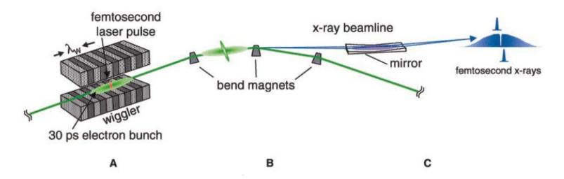
A Overlapping short laser beam with bunch center, meeting the resonance condition,
