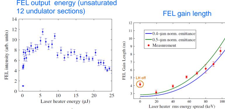
FIG. 15. (Color) FEL intensity at 1.5 Å measured on a downstream YAG screen vs LH energy when 12 undulator sections are inserted.
