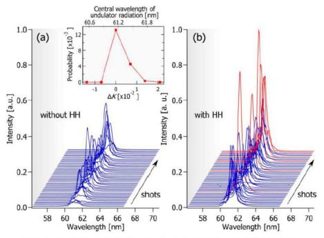
Fig. 2. Spectra of FEL radiation in fifty successive shots without (a) and with (b) HH injection. The red lines in (b) show profiles that have higher intensities above the threshold level. The inset shows an appearance probability of the high-intensity condition as a function of the deviation of K-value,  $\Delta K$ =K-1.37944 (lower axis), and the central wavelength of the undulator radiation (upper axis).
