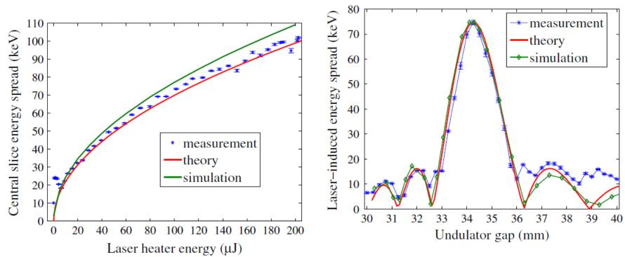
FIG. 8. (Color) Central slice rms energy spread vs LH energy.
