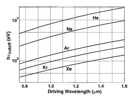
FIG. 1. Calculated relationship between single-atom HHG cutoff photon energy and the driving wavelength.
