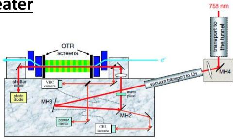
Align and match e-beam and laser beam using OTR screens
