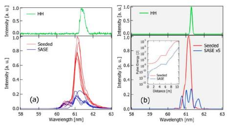
Fig. 3. Spectra of seeded (red lines) and unseeded (blue lines) conditions, as well as that of HH radiation (green line), given by experiment (a) and simulation (b). The inset of (b) shows intensity growths along the undulator for seeded (red line) and unseeded (blue line) conditions.
