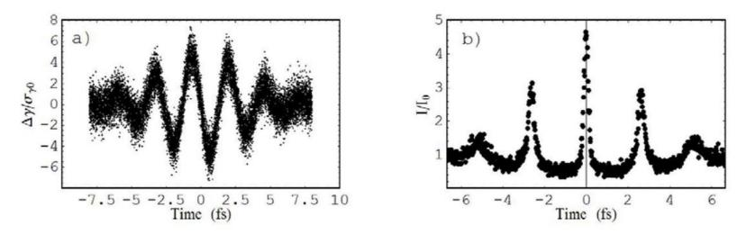
FIG. 5. Energy and peak current modulations produced in interaction with a few-cycle laser pulse. Only a part of the electron bunch affected by the interaction is shown.
