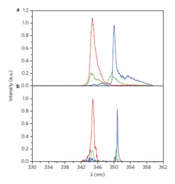
Figure 3 | Spectra for FEL radiation. a, Experimental results (red line, HGHG; blue line, EEHG; green line, intermediate state between HGHG and EEHG). b, Simulation results (red line, HGHG; blue line, EEHG; green line, intermediate state between HGHG and EEHG).
