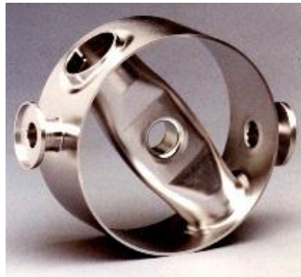
Prototype for ion beam acceleration 850 MHz, \beta=0.28 , 2-gap spoke cavity JLab
