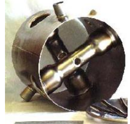
345 MHz, \beta=0.4 , 3-gap spoke cavity for ion beam acceleration ANL
