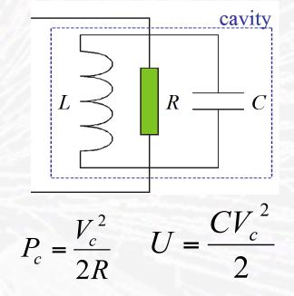
The voltage of the circuit is equivalent to a cavity voltage through a transit factor, V<sub>c</sub>=V<sub>0</sub> T
