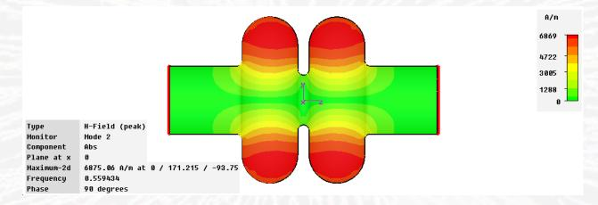
• A significant amount of power is dissipated in cavity walls and hence the cavities are heated, this must be water cooled in warm cavities and cooled by liquid helium in superconducting cavities. all power lost in the cavity must be replaced by an rf source
