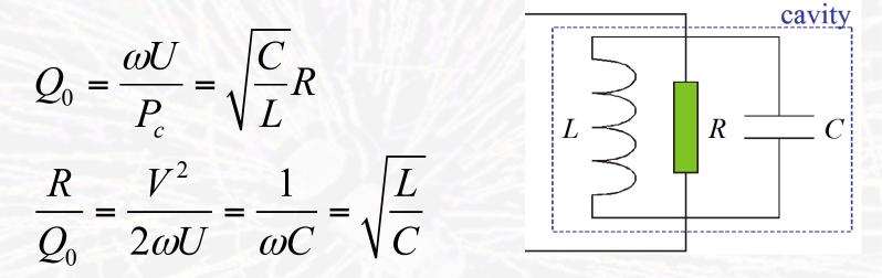
equivalent circuits have been proven to accurately model couplers, cavity coupling, micro-phonics, beam loading and field amplitudes including multi-cell cavities
