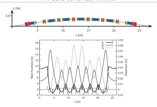
Note: vertical focusing provided by gradient in the bending magnets.
