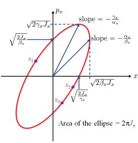
Applying simple geometry to the phase space ellipse, we find that the action (for uncoupled motion) is related to the Cartesian variables for the particle by:
