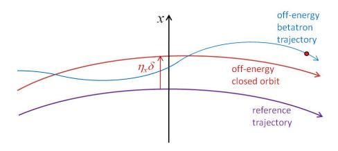
Coupling between transverse and longitudinal planes in a beam line is usually represented by the dispersion,  $\eta_x$ . So, in terms of the horizontal dispersion and betatron action, the horizontal coordinate and momentum of a particle are given by:
