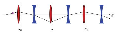
In an uncoupled periodic beam line, particles trace out ellipses in phase space with each pass through a periodic cell.
