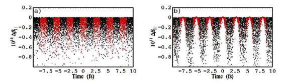
Figure 24. A distribution of the electron longitudinal velocities  $(10^{11}\beta)$  for unconditioned (a) and conditioned (b) electron beams. The uncorrelated energy spread of the particles is ignored.
