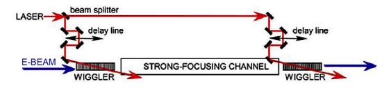
Figure 23. The laser conditioning scheme of Zholents is derived from the Vinokurov scheme.
