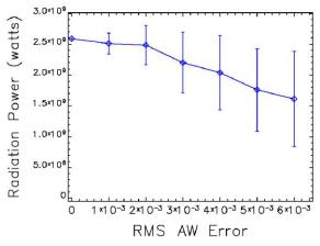
Figure 18. Output radiation power at 40-nm from FEL-1 of FERMI produced by random undulator segment mistuning as a function of RMS error in a<sub>w</sub>. The diamond symbol and error bars refer to the mean and standard deviation over 64 independent mistunings. The distribution of errors at individual segments follows a one-dimensional Gaussian.
