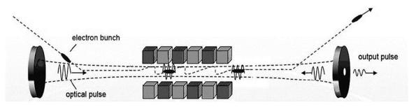
Figure 19. Simplified schematic of a cavity FEL
