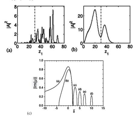
Figure 8<sup>37</sup>. Numerical solutions 1-D FEL field equations in the classical and quantum regimes: Graphs (a) and (b) show the scaled field intensity  $|A|^2(z_1)$  after 50 gain lengths when the system evolves classically  $\rho' = 5$  and quantum mechanically  $\rho' = 0.05$ , respectively.  $z_1$  is the retarded time. Graph (c) The imaginary part of the unstable root of the cubic equation v.  $\overline{d}$ ; for  $1/\overline{r} = 0$ ; (a) 0.5, (b) 3, (c) 5, (d) 7, (e) and 10, (f).
