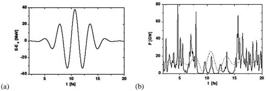
Figure 12 (a) Energy modulation of the electron beam at the exit of the modulator undulator. The laser parameters are wavelength = 800 nm,  $W_{peak}$  = 800 GW, and FWHM pulse duration of 5 fs. (b) Typical single-shot temporal structure of the central part of the radiation pulse. Undulator length is 120 m. Dotted line shows energy modulation of the electron bunch shown in panel (a).
