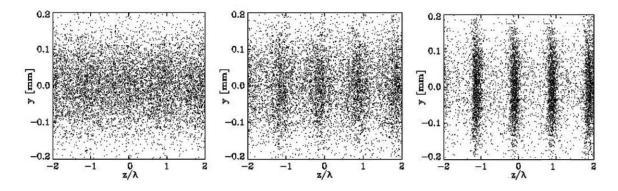
Figure 4. GENESIS calculations of particle positions in the transverse direction y and in z at three locations along the undulator. Left panel is at the entrance to the undulator; the right panel is at saturation. The central panel is at an intermediate position.
