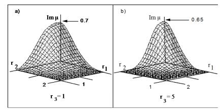
Figure 6. Gain surface, Im  $\mu$ , versus scaled emittance and energy spread for two values of the diffraction parameter,  $r_3$
