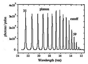
Figure 17. HHG spectrum of Ne from the 35<sup>th</sup> to 59<sup>th</sup> harmonic
