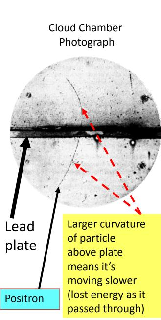
A "Cloud Chamber" is capable of detecting charged particles as they pass through it.
