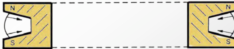
Cross section of weak focusing circular accelerator
