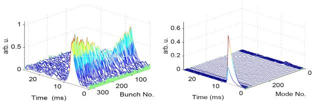
The plots above show measurements made at the ALS, revealing coupledbunch modes driven by the resistive-wall wake field.
