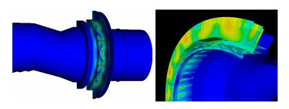
Calculation of trapped modes in PEP II bellows. Higher-order mode heating is a significant problem for PEP II, and a potential problem for the ILC damping rings. (Cho Ng, SLAC).
