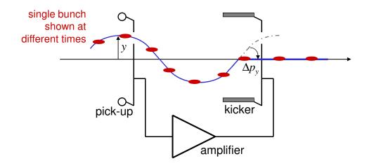
An ideal feedback system will detect the position of a single bunch, and apply a kick that immediately restores the bunch to its correct trajectory.
