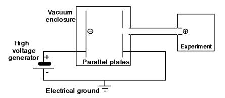
Figure 1. The DC accelerator
