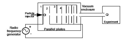
Figure 3. A multi-cavity radio frequency accelerator
