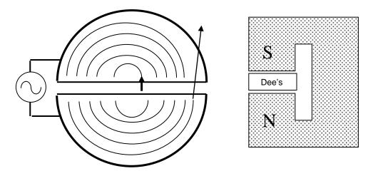
Figure 6 The cyclotron : top view (left) and side view (right)
