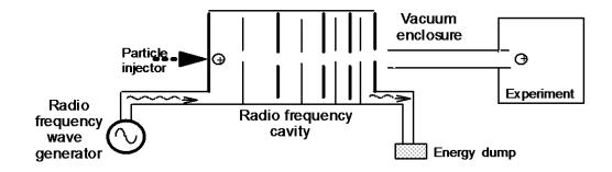
Figure 4. Accelerator with rf-cavities
