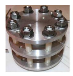
Fig. 4. Photograph of Two-Switch Electrode assembly.
