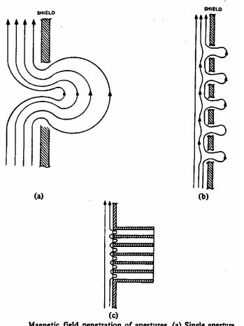
Magnetic field penetration of apertures. (a) Single aperture. (b) Many small apertures. (c) Array of waveguides beyond cutoff. •Screen boxes can be used to reduce coupling to diagnostics and equipment
