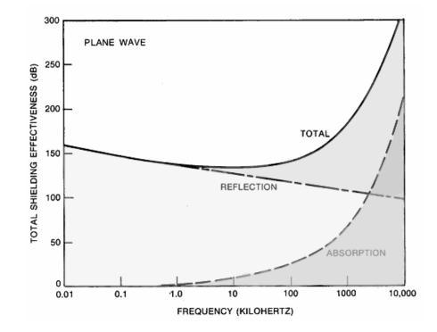
Method of shield effectiveness depends on frequency range -At low frequency, most incoming radiating is reflected -At higher frequency, absorption becomes more dominant
