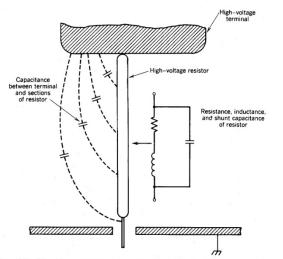
Figure 9.51 Effect of stray capacitance, shunt capacitance, and series inductance on resistive voltage divider.
