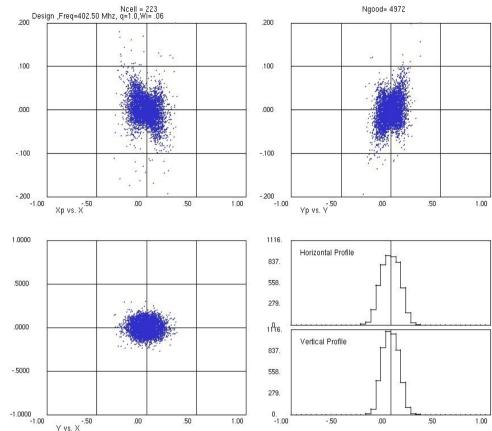
The plot on the left shows the longitudinal phase space (energy vs. phase), along with the surrounding separatrix. Also plotted is again the x-y distribution and histograms of the energy and phase distribution for cell 437 of the SNS RFQ, near the end.
