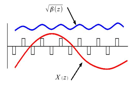
Each ray is the product of the two functions. Chapter 7 Radio Frequency Quadrupole
