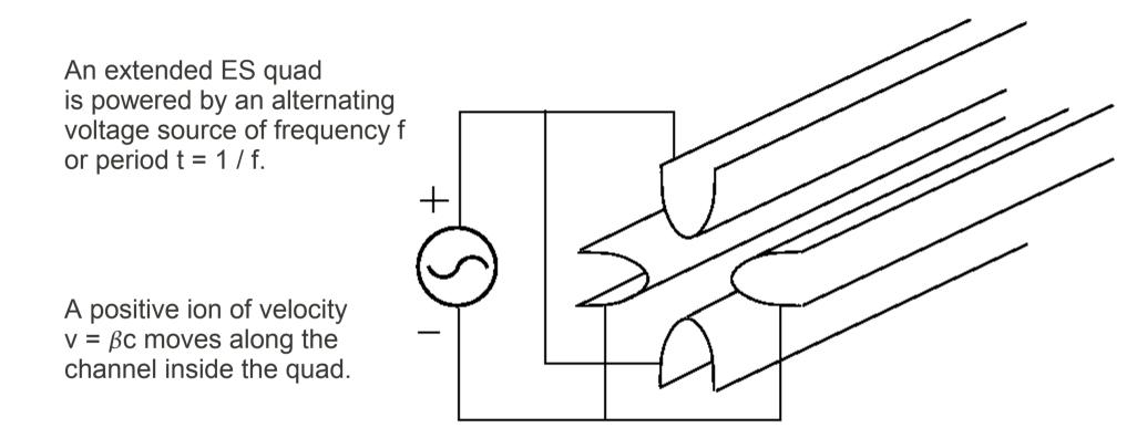
The quadrupole field along the axis will vary as  $\cos(\omega t)$ ,  $\omega = 2\pi f$
