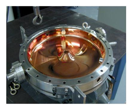
The interior of the pillbox rebuncher cavity (one-half shown) operates in the  $TM_{010}$  mode at 402.5 MHz. The gap voltage is about 65 kV. Twelve quadrupoles provide transverse focusing. In the jaws of several of the quadrupoles is a beam position monitor (in front of the quadruple) that provides beam position, intensity and timing information.
