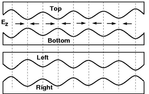
The tips of the poles (vanes) in the RFQ are modulated with wiggles, where the phase of the wiggles in the top and bottom vanes is out of phase of those in the left and right vanes.
