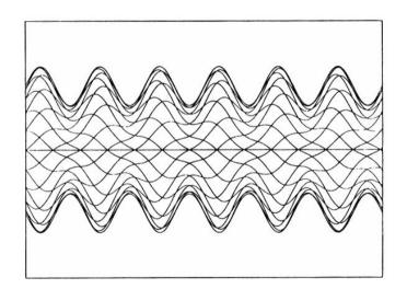
The beam is the ensemble of all the rays within the envelope.
