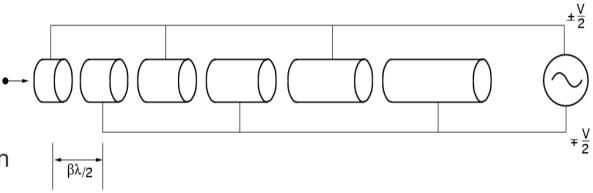
In a typical proton accelerator system, a 50-100 kV ion source will inject an RFQ, which will accelerate the beam to 2-3 MeV, followed by a drift-tube linac, further accelerating the beam to 100-200 MeV, at which point the drift-tube linac efficiency is lower than a more efficient structure, such as a side-coupled linac.
