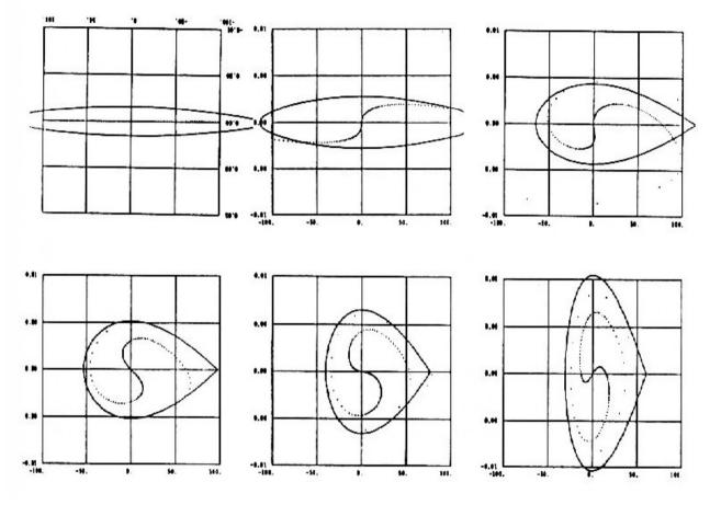
(phase) length during the bunching process. After several phase oscillations, the majority of the injected beam is concentrated near the center of the separatrix.
