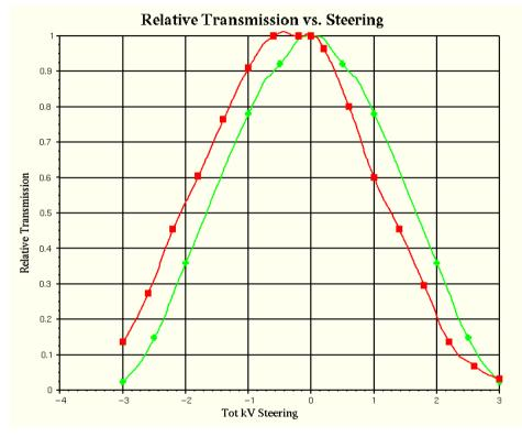
Many other parameters may be calculated, such as the transmission as a function of transverse offset of the beam at the entrance of the RFQ. Here, the measured transmission shows excellent agreement, but with a steering offset error.
