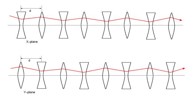
For certain values of the focusing/defocusing strengths and the distance between elements, a stable transport solution exists.
