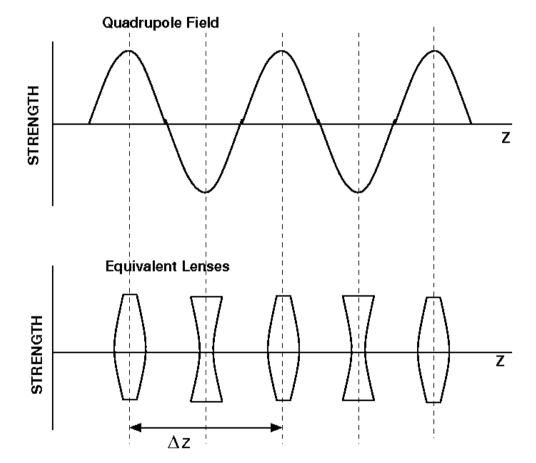
The alternating field electrostatic quadrupole acts like a strong focusing sequence.
