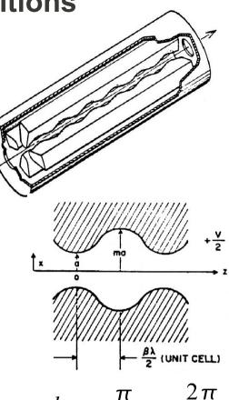
$$\left(\frac{a}{r_0}\right)^2 + A I_0(ka) = 1, \quad \left(\frac{ma}{r_0}\right)^2 - A I_0(mka) = 1, \quad k = \frac{\pi}{L_c} = \frac{2\pi}{\beta\lambda}$$
