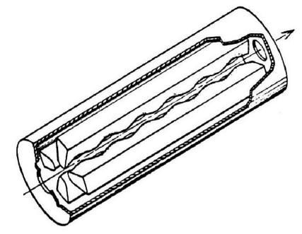
The 4-rod RFQ is generally used at frequencies of 200 MHz on down. It is non-symmetric, requiring more attention to thermal expansion issues, but has a simpler mode structure.
