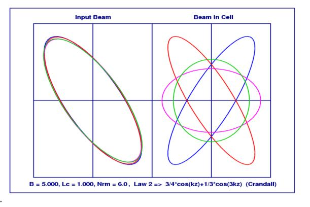
The transformation from a steady beam to one where the envelope is matched to the time-varying RF field takes place in the radial matcher (RM). The RM is typically about 6 cells long, and the radius of the RFQ vanes starts at a large value and tapers down to the final radius from the axis  $r_0$  in the unmodulated vane.
