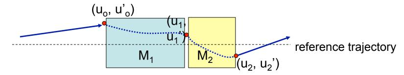
The solution for the first element becomes the initial condition for the second element...
