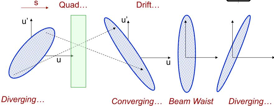
A focusing quadrupole causes a diverging beam to converge. In reality, the scenario is more complicated because we focus in one plane while defocusing in the other.
