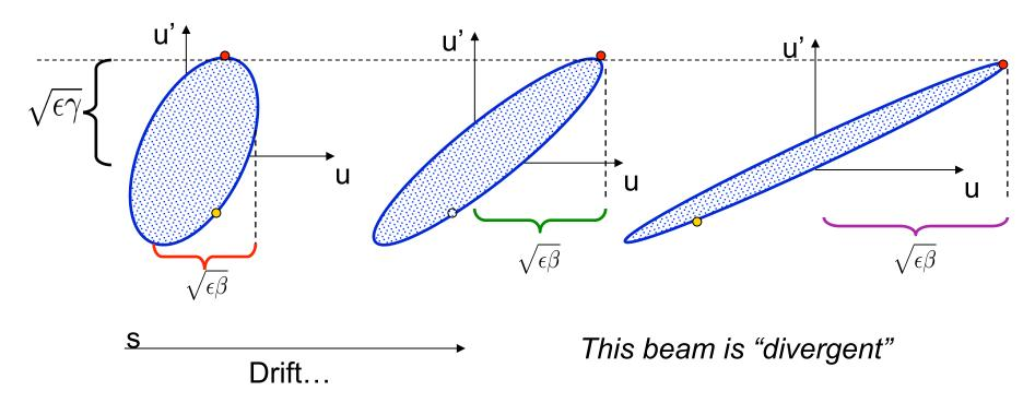
Analogous to a single particle, u increases while u' remains fixed. Observation: Without focusing, any beam would spread out...
