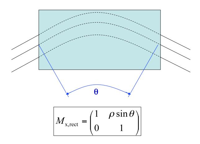
In the horizontal direction the magnet transforms like a drift with length equal to the path length  $\rho$  sin  $\theta$ .
