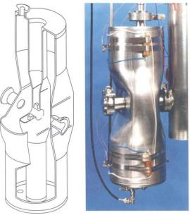
**Figure 4.26** 350-MHz  $\beta = 0.12$  coaxial half-wave resonator with a single loading element (courtesy of J. R. Delayen, Ref. 33).
