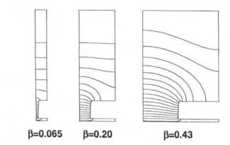
Figure 4.9 Electric-field lines shown in one quarter of the projections of three DTL cells as calculated by the program SUPERFISH (courtesy of J. H. Billen).
