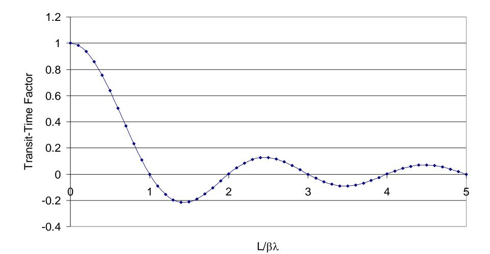
For efficient acceleration by RF fields, we need to properly match the gap length *L* to the distance that the particle travels in one RF wavelength,  $\beta\lambda$ .
