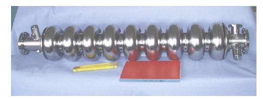
Superconducting RF cavity for ILC
