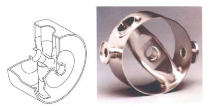
**Figure 4.27** 850-MHz,  $\beta = 0.28$  spoke resonator (courtesy of J. R. Delayen, Ref. 33).
