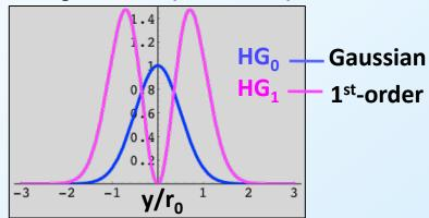
Allows additional (independent) control of focusing forces (and matched beam spot)
