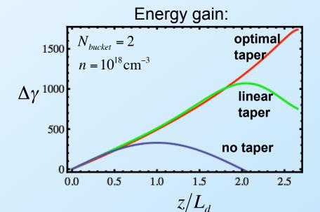
In plasma channel, focusing and accelerating wakes have different phase velocities: varying density and channel radius to phase lock both.
