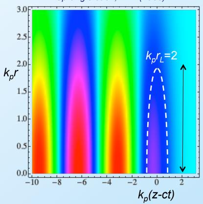
Wakefields determined by local laser intensity gradient: extend to laser spot  $\sim r_L$
