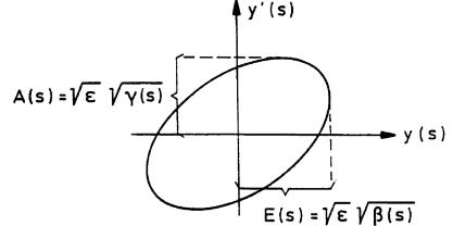
Beam envelope E(s) and divergence A(s). Note also  $\gamma(s) = (1 + \alpha^2(s)) / \beta(s)$
