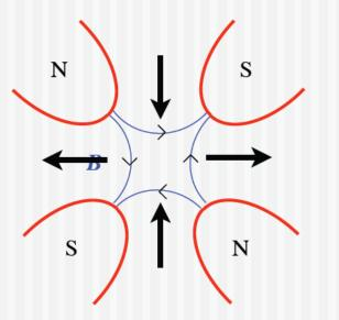
Because of the v x B term in  $\vec{F} = ma = e(\vec{E} + \vec{v} \times \vec{B})$
