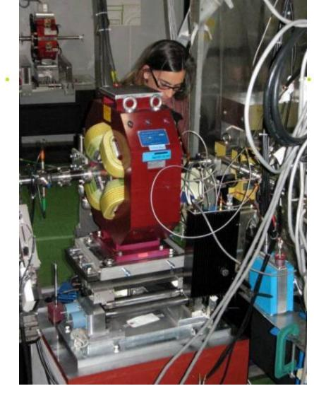
T.Smith is commissioning the cavity BPM electronics and the magnet mover system at ATF beamline
