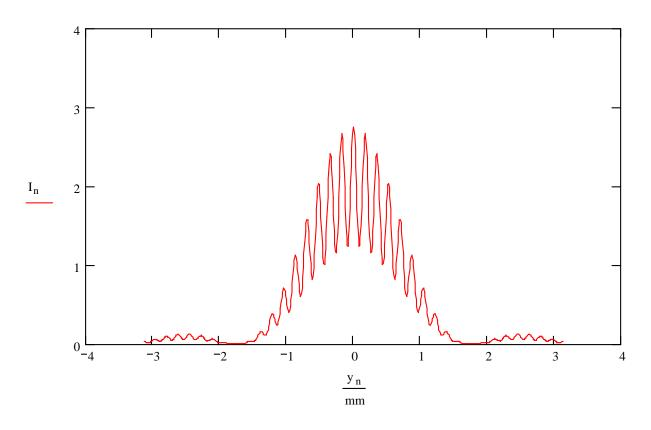
Fringe pattern of an extended source, with  $\sigma_0$ =0.2 mm
