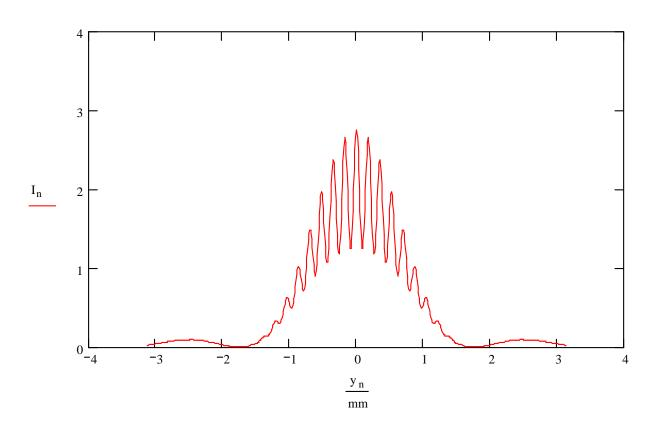
Fringe pattern using a Gaussian bandpass filter with a full width at half maximum (FWHM) of  $\Delta \lambda = 30$  nm.
