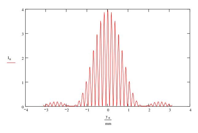
Fringe pattern of a monochromatic point source at 450 nm, using parameters for the PEP-II HER interferometer at SLAC.  $A_1 = A_2 = 1$ , d = 5 mm, a = 0.5 mm.
