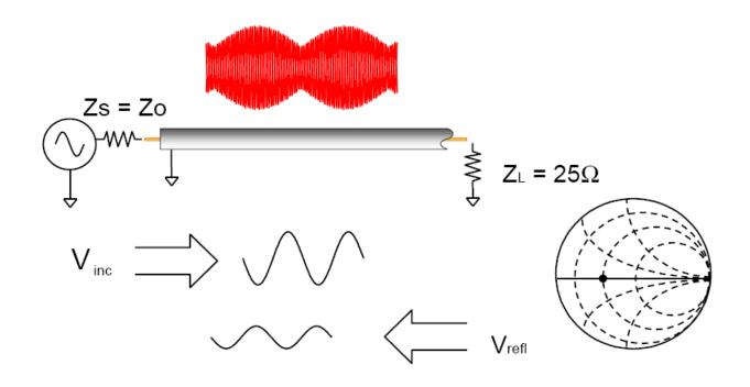
Standing wave pattern does not go to zero as with short or open
