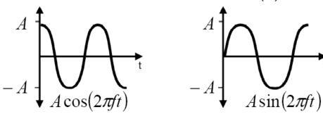
The phasor's x and y axis projections, as a function of time, map out cosine and sine waves, respectively
