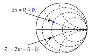
At high frequencies, maximum power transfer occurs when  $R_S = R_L = Z_0$
