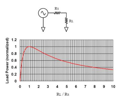
Maximum power is transferred when  $R_L = R_S$
