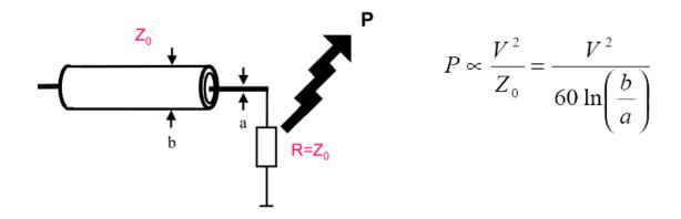
Power efficiency will be limited by the electric field between the 2 conductors
