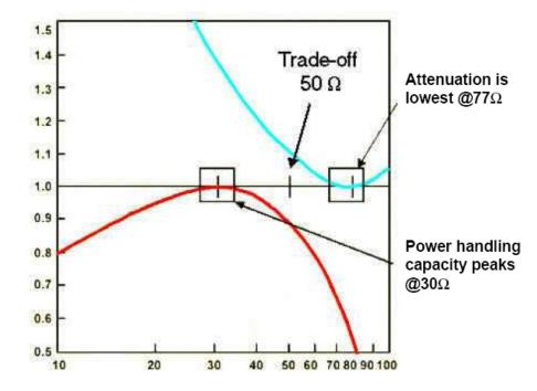
Characteristic impedance for coaxial airlines  $(\Omega)$
