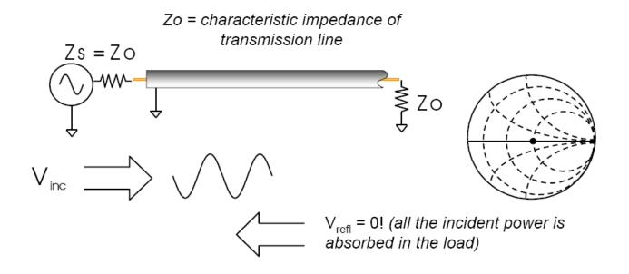
For reflection, a transmission line terminated in Zo behaves like an infinitely long transmission line
