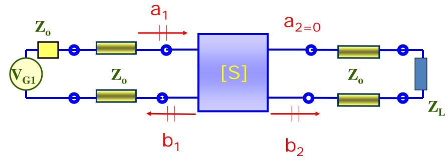
Measurement of  $S_{11}$  and  $S_{21}$  by matching the line impedance  $Z_{\circ}$  at port 2 through a corresponding load impedance  $Z_{L}=Z_{\circ}$
