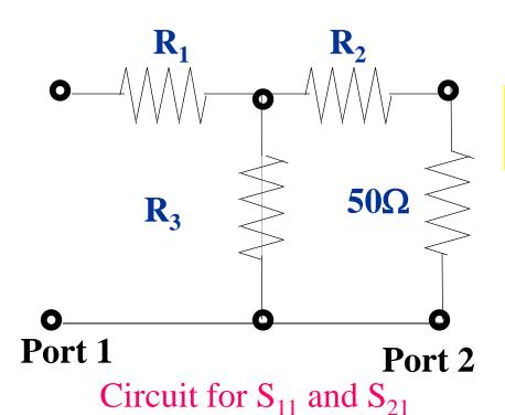
$$Z_{in} = R_1 + \frac{R_3(R_2 + 50\Omega)}{(R_3 + R_2 + 50\Omega)} = 50\Omega$$
