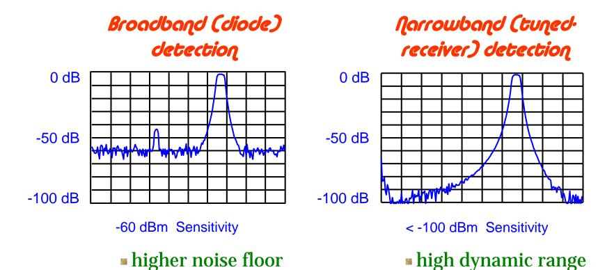
Dynamic range = maximum receiver power - receiver noise floor
