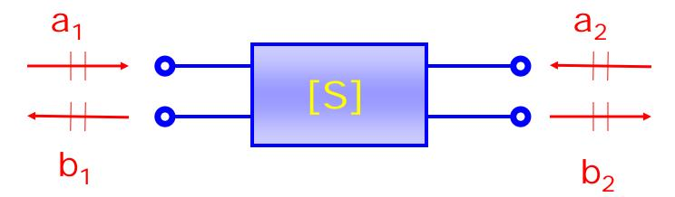
a<sub>n</sub> – normalized incident power waves
