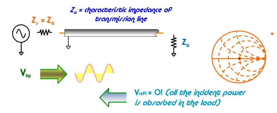
For reflection, a transmission line terminated in Zo behaves like an infinitely long transmission line
