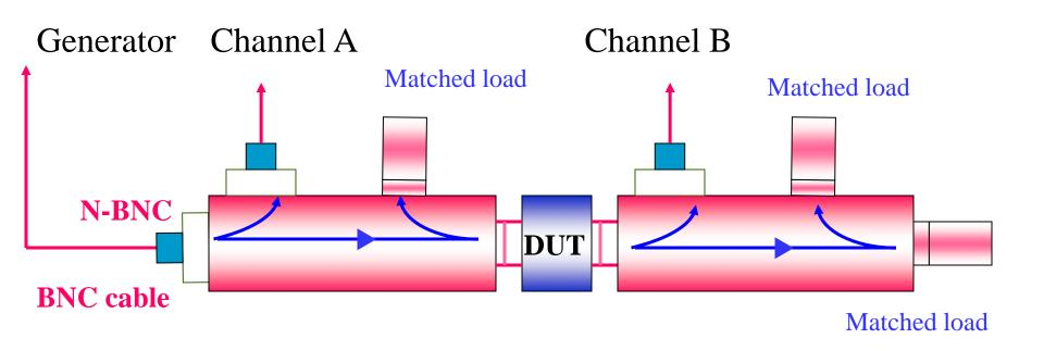
The DUT is connected directly between two directional couplers. Voltage at A of the VVM is proportional to the voltage wave incident on the DUT while the voltage at B of the VVM is proportional to voltage wave transmitted through the DUT.
