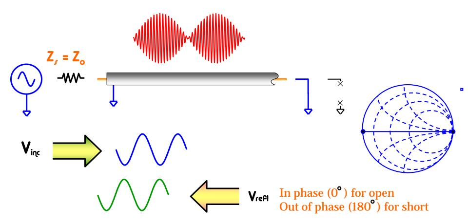
For reflection, a transmission line terminated in a short or open reflects all power back to source
