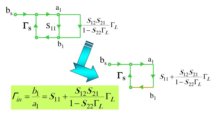
Note: Only  $\Gamma_L = 0$  ensures that  $S_{11}$  can be measured.
