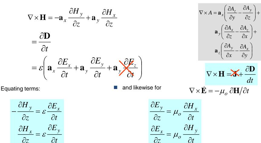
Spatial rate of change of H is proportionate to the temporal rate of change of the orthogonal component of E & v.v. at the same point in space
