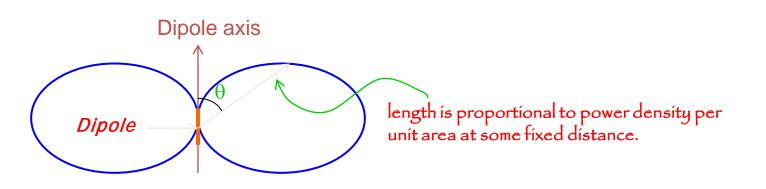
Note: No radiation takes place along the dipole axis, and the radiation pattern has axial symmetry, with maximum radiation being in the equatorial plane.
