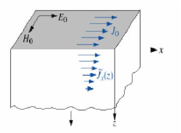
Current density decays exponentially from the surface into the interior of the conductor
